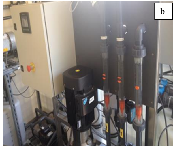
Figure 2. Presentation of the pilot system (a) the compact unit containing (from the left to the right) the MBR, aeration, anoxic and equalization tanks, (b) the RO unit.
