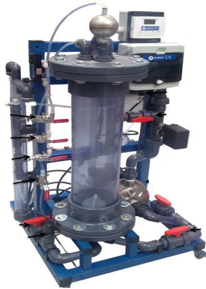
Figure 24: Ozone disinfection pilot
