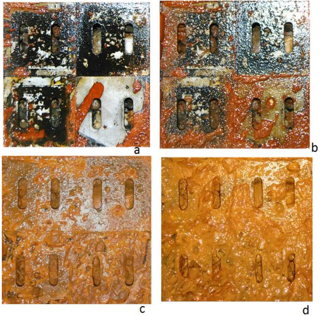
Figure 8: Evolution of the column well screen clogging after 1(a), 20(b), 29(c) and 73(d) days
