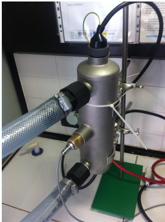
Figure 28: UV Reactor used in the experiment
