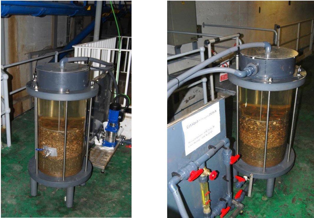
Figure 4: Water injection pilot located next to the sand-filtered water canal of SJD DWTP
