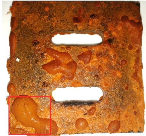
Figure 12: Metallic piece of the well screen simulation with biofilm material deposition
