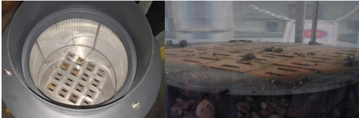
Figure 6: Picture of the well screen simulation in the column experiment NOTE: Left picture: before starting. Right picture: at the beginning of the operation
