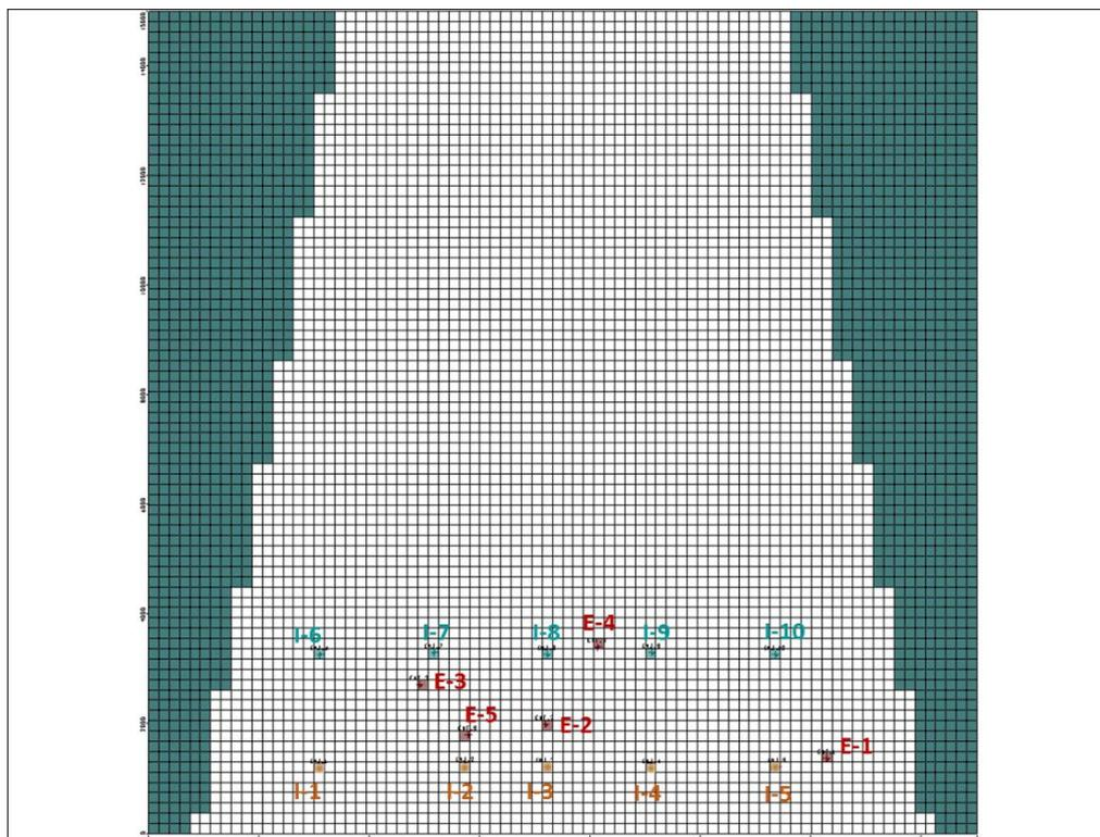
Figure 10: Location of wells (E: extraction, and I: injection) in the model
