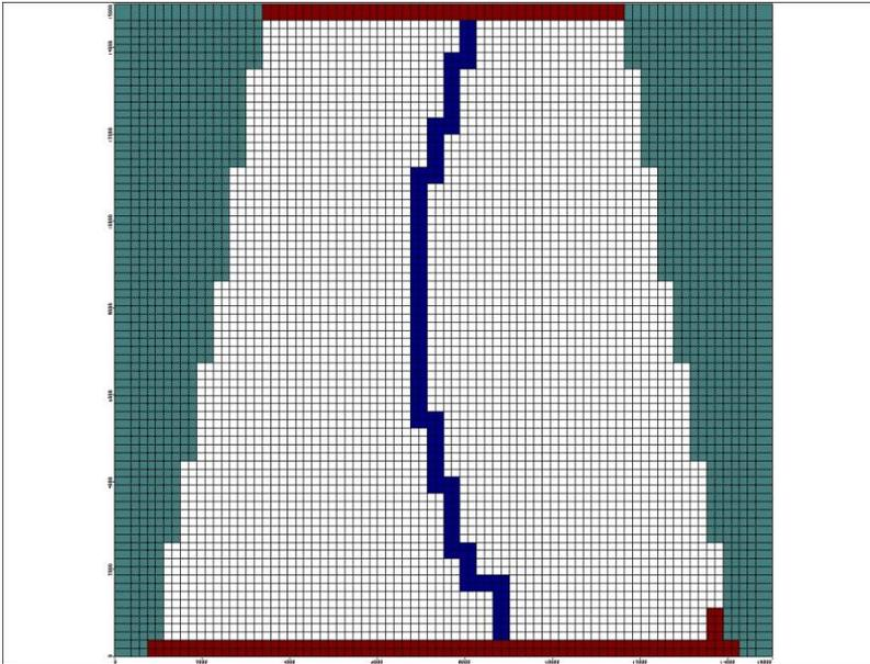
Figure 12: Boundary conditions. River boundary condition (blue), upstream constant head boundary condition and downstream or sea coastline boundary condition (brown). Green cells are not activated and the contact of these green cells with the aquifer is of no flow boundary condition.
