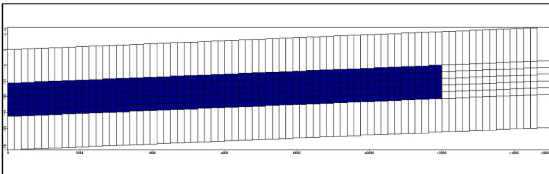
Figure 11: Cross-section of the aquifer. Aquitard materials are indicated in blue color while shallow and depth aquifer are in white color.
