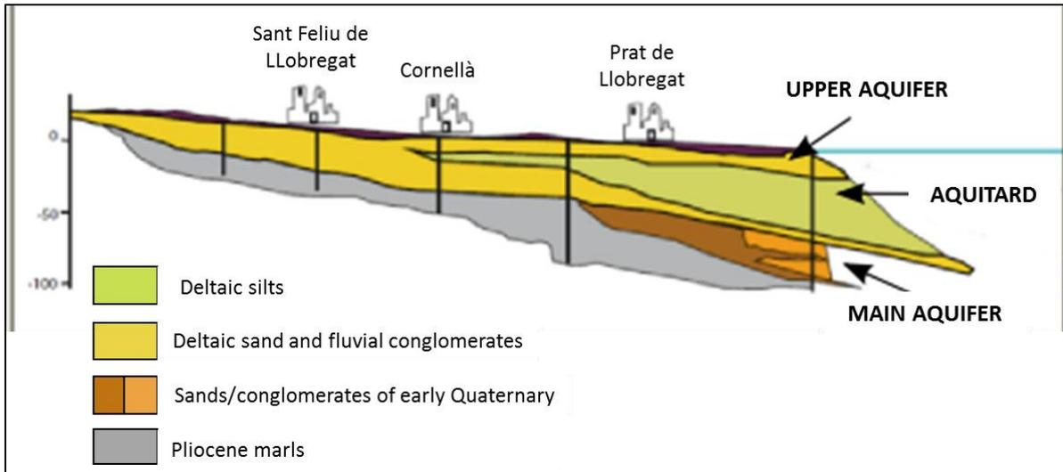
Figure 3: Cross section of Llobregat Delta Aquifer (MOP, 1966, Manzano et al , 1992; modified by UPC, 2002).
