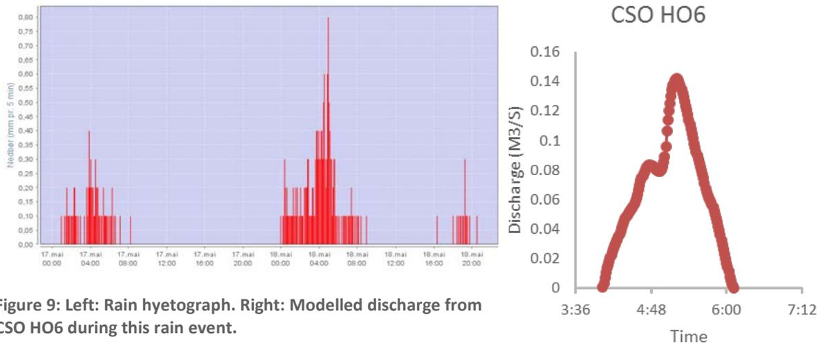
Figure 9: Left: Rain hyetograph. Right: Modelled discharge from CSO HO6 during this rain event.
