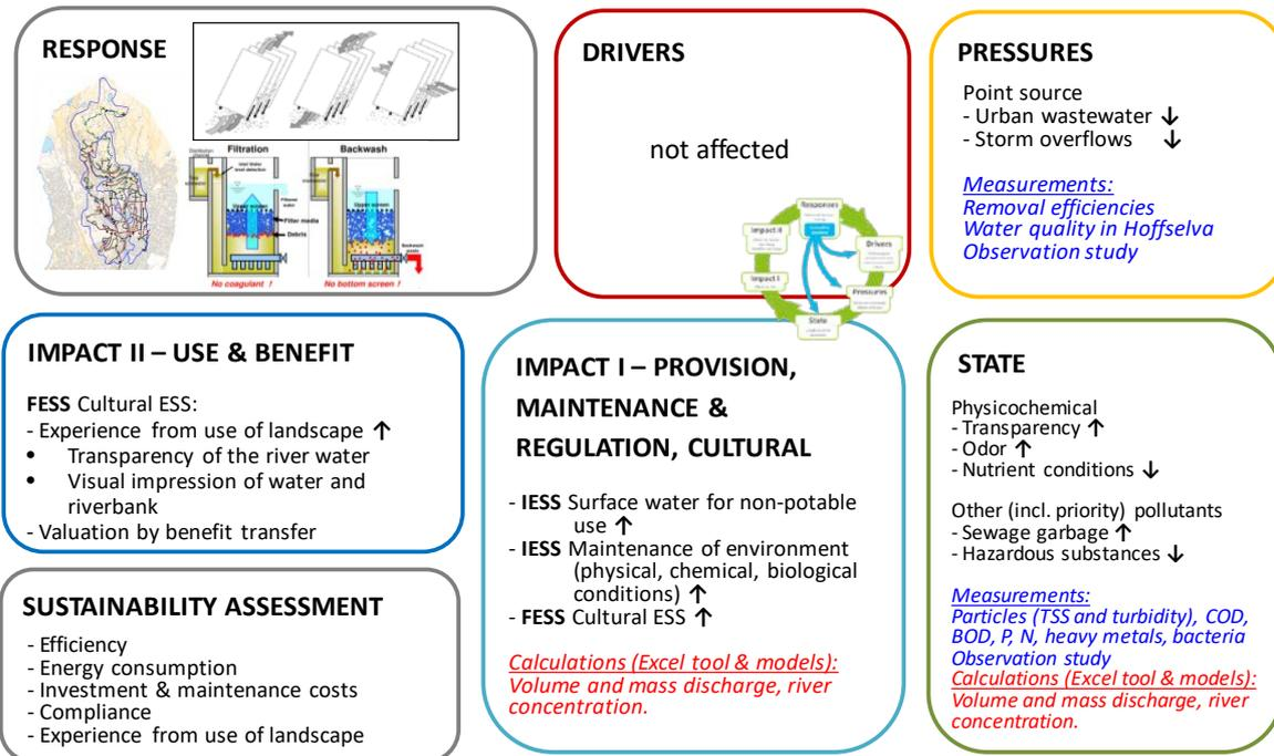
Figure 1: Overview graphic of Hoffselva demo case “Decentralised water treatment”.
