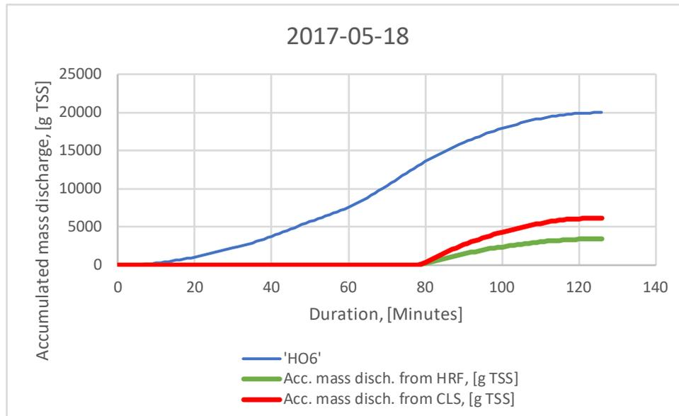
Figure 4: Simulated mass discharge from the CSO "HO6" during the rain event of 2017-05-18. The blue line shows the mass discharge without any treatment. The red and green lines show the combined effect of the chosen storage volume (339 m<sup>3</sup>) and the CLS and HRF solutions, respectively.
