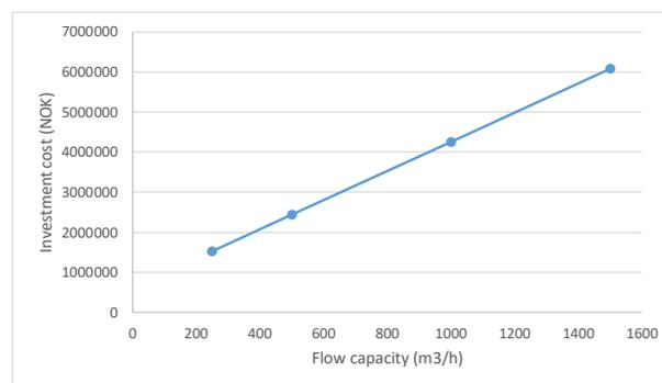
**Figure 17 Correlation between flow capacity and CLS plant investment cost**
