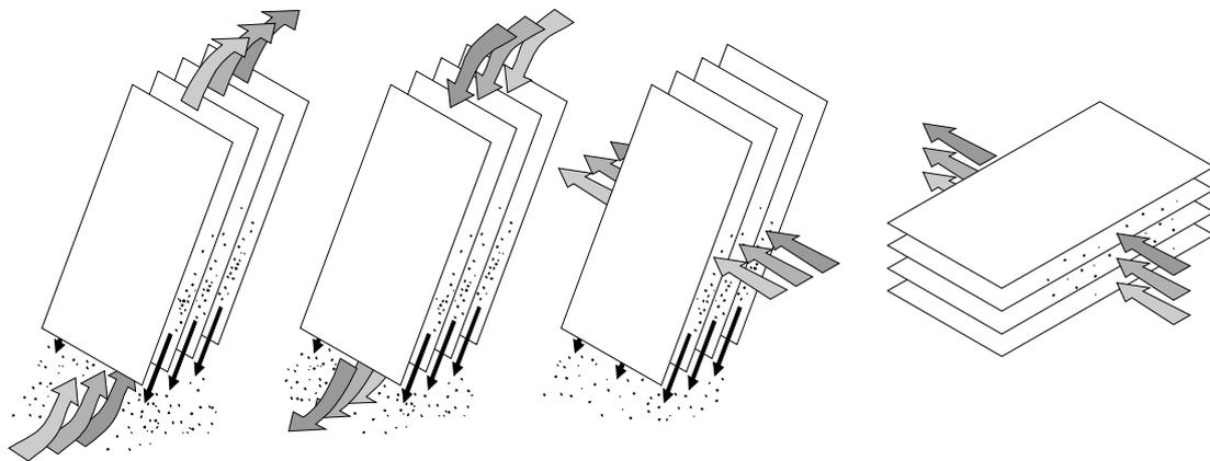
**Figure 3 Up-flow, down-flow, cross-flow and horizontal plate lamella settlers**
