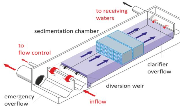
Figure 14: CLS settler installed in underground container
