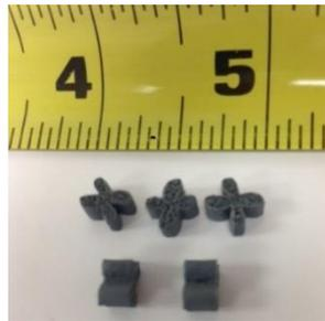
Figure 1 Special designed media of HRF
