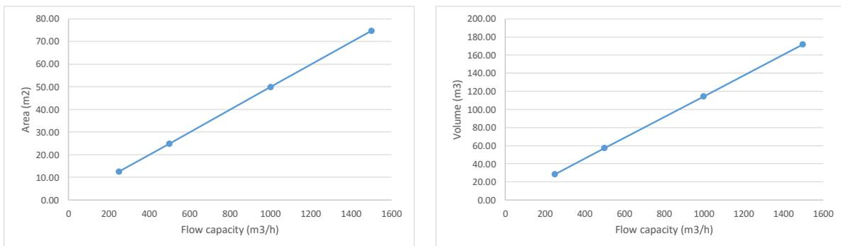
Figure 15 Correlation between flow capacity and CLS plant dimension (area and volume)
