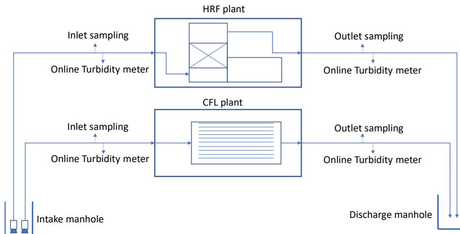
Figure 7 Diagram of HRF and CLS demonstration plants
