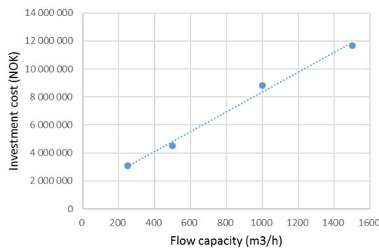
**Figure 13 Correlation between flow capacity and HRF plant investment cost**
