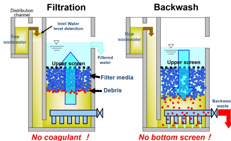
Figure 2 HRF system process diagram
