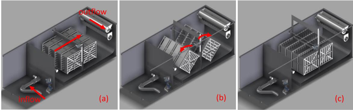
Figure 4 CLS process diagram (a) flow direction, (b) Lamella pivots under water for cleaning, (c) Lamella in vertical position, allowing settling of sludge
