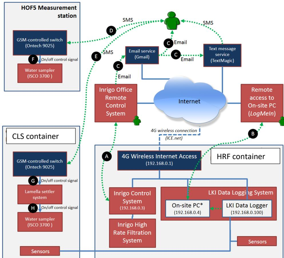
Figure 8 Communication system architecture of demonstration plants
