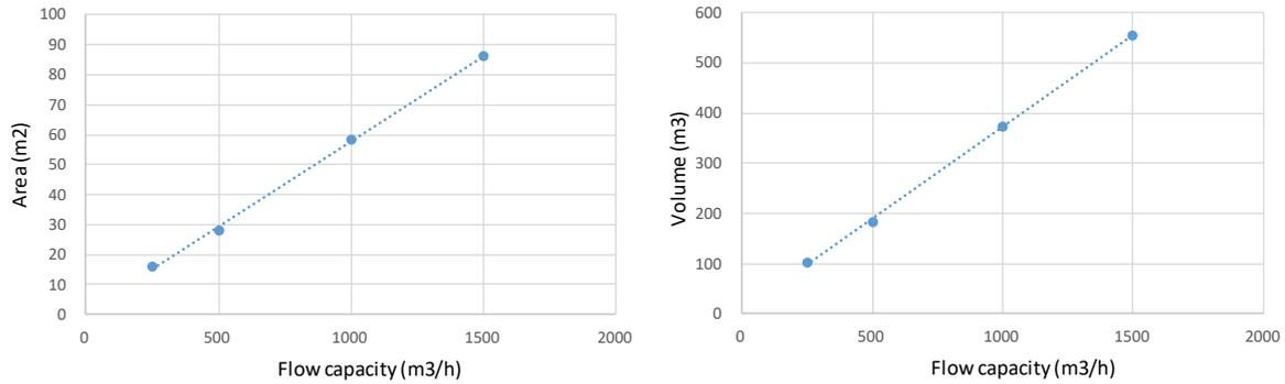
**Figure 12 Correlation between flow capacity and HRF plant dimension (area and volume)**
