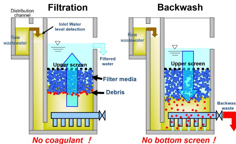
Figure 2 HRF system process diagram
