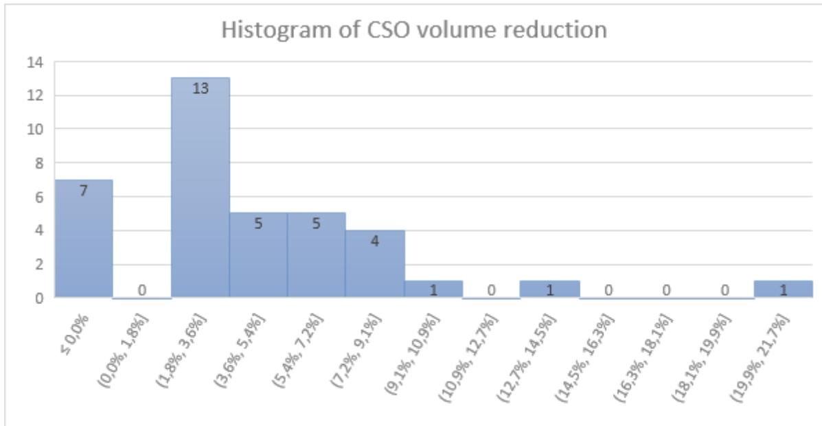
Figure 87 Frequency of reduction rates (regarding overflow volume) (%) for the 37 tanks in the catchment with ADESBA compared to the system without ADESBA.
