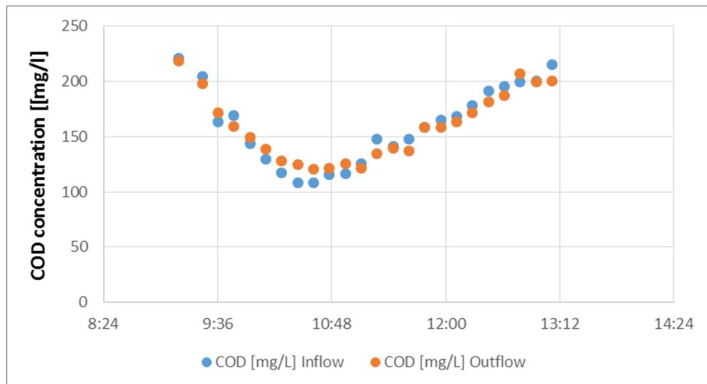
Figure 50 COD concentration during an exemplary dry weather test without lamellae with a flow of 10 l/s.
