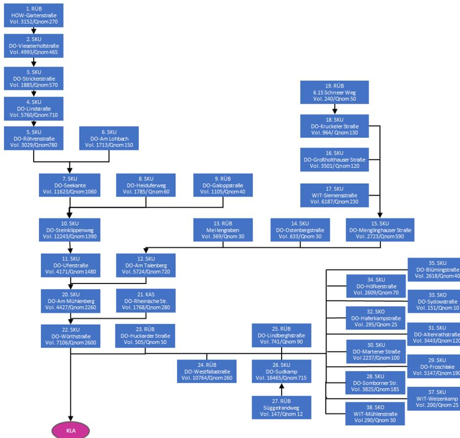
Figure 83 Sewer network of the whole sub-catchment of the WWTP Dortmund Deusen.
