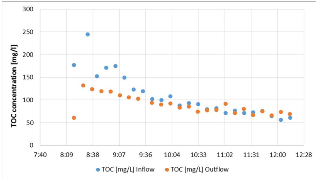
Figure 37 TOC concentration during an exemplary dry weather test with a flow of 10 l/s (corresponding to a surface loading in the container of 1.1 m/h).
