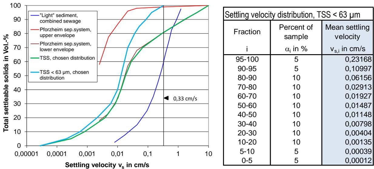
Figure 4 Distribution of settling velocity for different types of sediment and for TSS fine fractions in surface runoff of separate systems (Weiss 2016).
