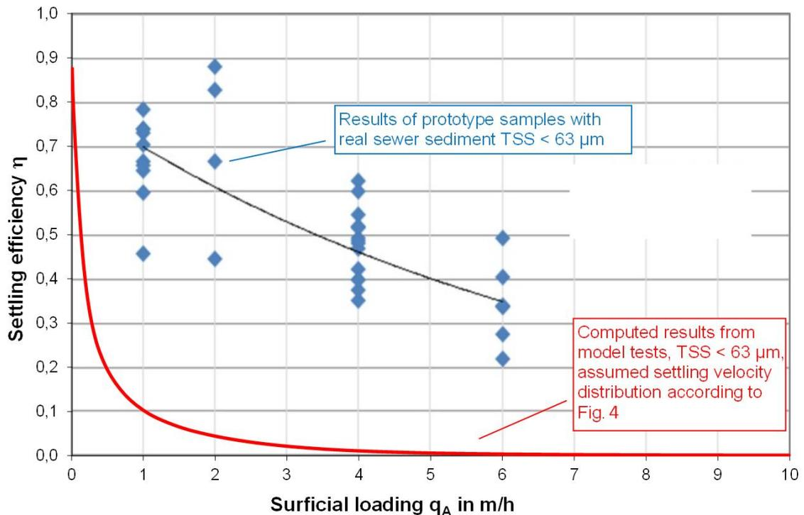
Figure 3 Comparison of measured settling efficiencies of real sewer sediment (TSS < 63  $\mu\text{m}$ ) to computed values from model tests (Weiss 2016).
