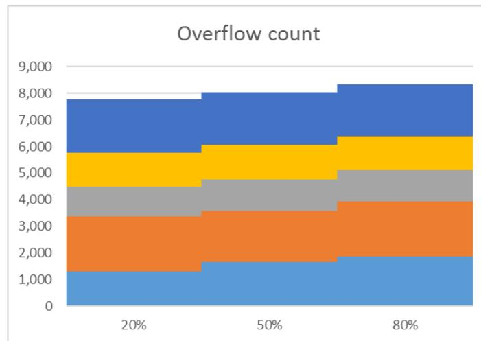
**Figure 68** Total overflow count resulting from the Simba# simulation with ADESBA in place. The throttle range in which ADESBA operates was varied from 20 to 50 to 80% of the total range between zero and Qmax. The simulations are based on 25 year MOMENT data. Different colours indicate overflow volume share of each CSO facility.
