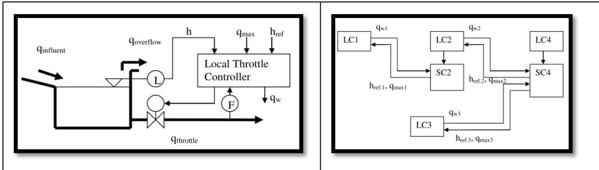
Figure 61 RTC structure of ADESBA using local (LC) and supervisory (SC) controllers (Alex *et al.* 2008).
