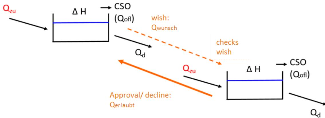
Figure 56 The upper basin sends a wish for a throttle setting to the lower basin, which checks the wish in relation to its own water level.  $\Delta H$  = water level,  $Q_{zu}$  = Inflow,  $Q_d$  = throttled outflow, CSO ( $Q_{ofl}$ ) = overflow,  $Q_{wunsch}$  = desired throttle setting,  $Q_{erlaubt}$  = approved throttle setting.
