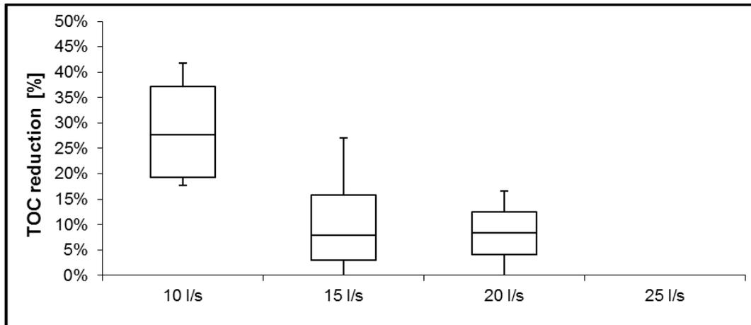
Figure 44 Reduction range for parameter TOC at different flow rates.
