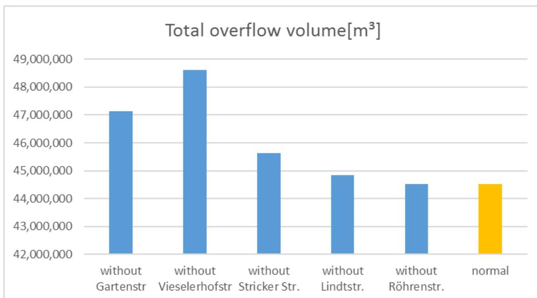
**Figure 70** Total overflow volume (m<sup>3</sup>) simulated with ADESBA based on 25 year MOMENT data. Single tanks were excluded from the ADESBA control.
