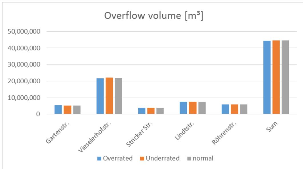
Figure 72 Overflow volume (m<sup>3</sup>) resulting from Simba# simulation with normal/“real” and over- and underestimated water-level-to-storage-volume relationships at Vieselerhofstr.
