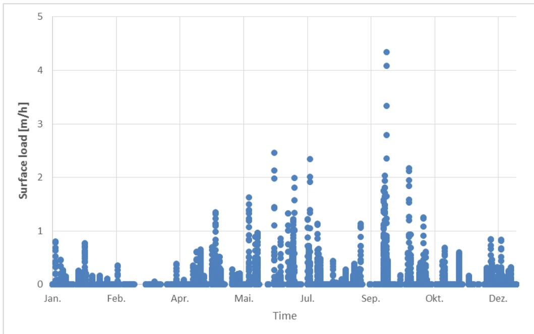
Figure 51 Theoretical surface loads (m/h) at CSO Gartenstraße according to inflow rates over one year (2014) with 50 % of the storage volume equipped with lamellae. One data point represents the surface load resulting from the given lamella surface and the inflow simulated in the MOMENT model every five minutes.
