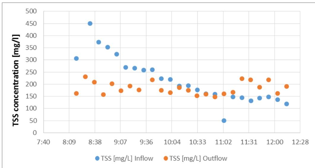
Figure 34 TSS concentration during an exemplary dry weather test with a flow of 10 l/s.
