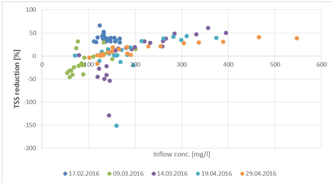
Figure 45 Concentration of TSS in the inflow and reduction on the way to the overflow for five test runs with dry weather at a flow rate of 10 l/s.
