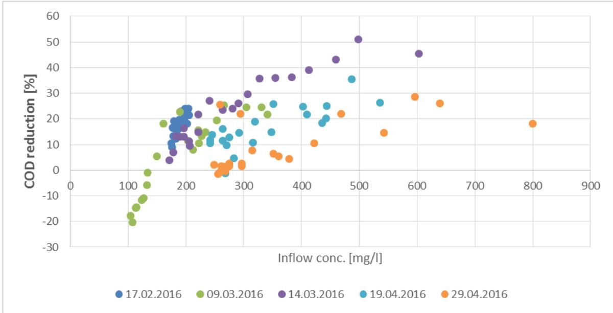
Figure 47 Concentration of COD in the inflow and reduction on the way to the overflow for five test runs with dry weather at a flow rate of 10 l/s.
