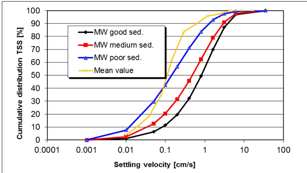
Figure 31 Mean settling velocity of sediments in three dry weather sample (yellow) in comparison to literature results of combined sewage samples with poor (blue), medium (red) and good (black) sedimentation behaviour.
