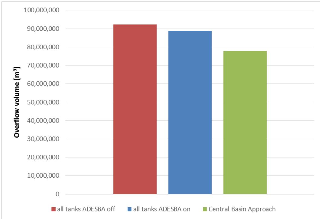
Figure 88 Total overflow volumes for a 10 year period. Results for the whole catchment with and with ADESBA are compared to the central basin approach (theoretical optimum).
