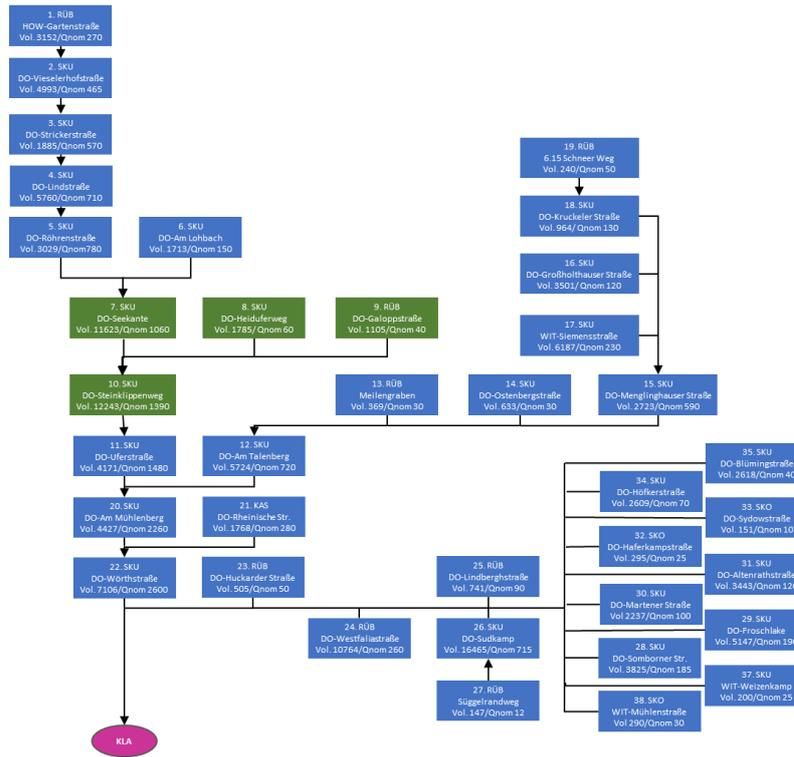
Figure 91 Example of tank combination no. 15 for real time control within the sub-catchment of the WWTP Dortmund Deusen. Green tanks are selected for control with ADESBA.
