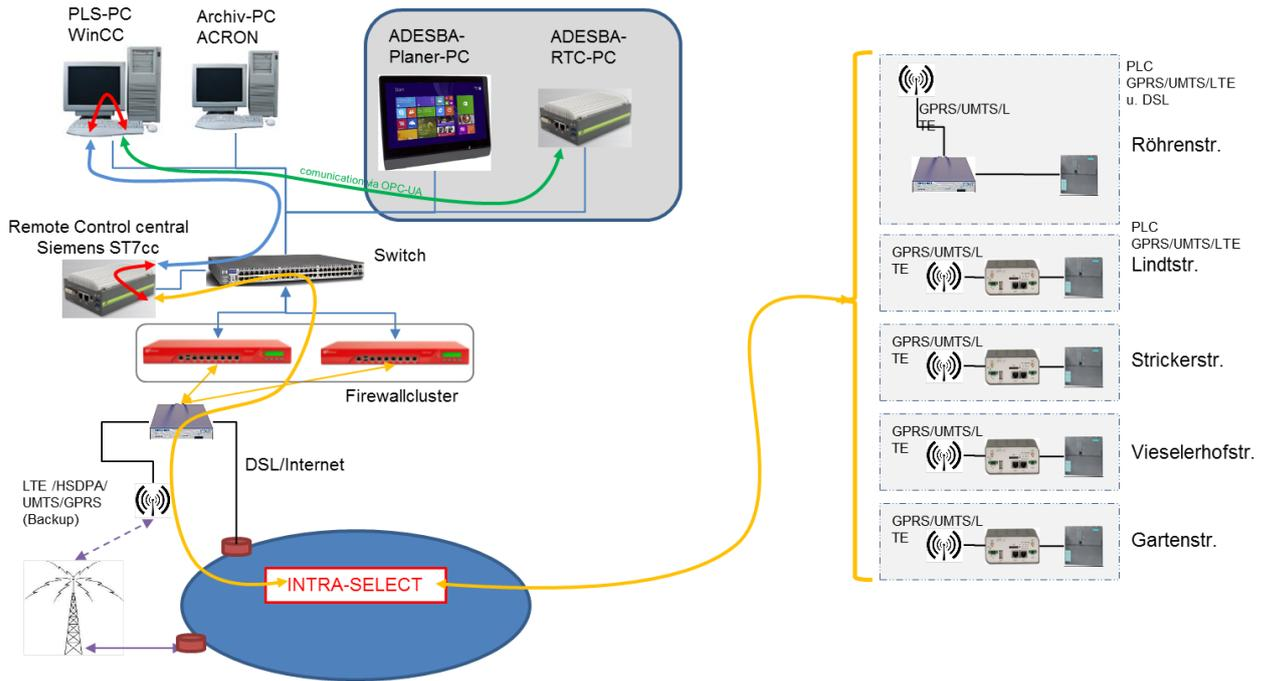
Figure 74 Communication and data transfer scheme for RTC implementation at the five CSOs.
