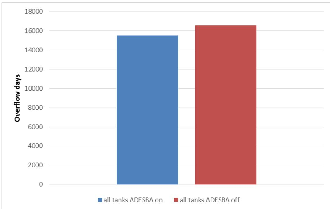
Figure 89 Total overflow days for a 10 year period. Results for the whole catchment with and with ADESBA control.
