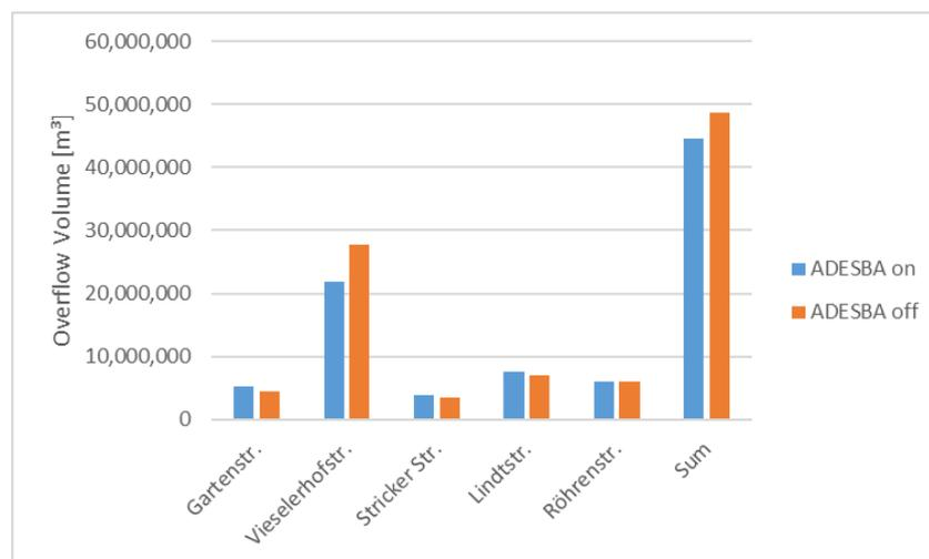
Figure 63 Overflow volume for each CSO facility and summed up overflow volume of all five facilities calculated in Simba# with and without ADESBA.
