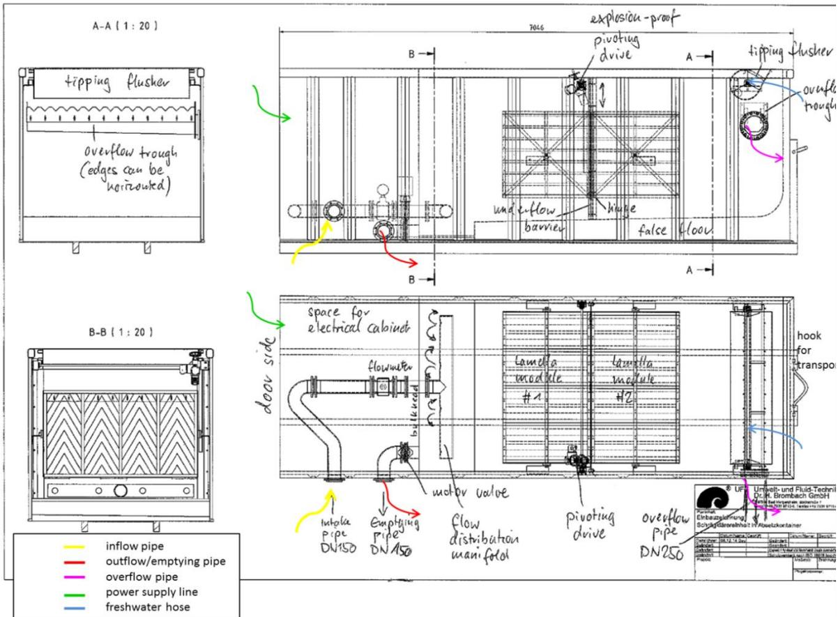
Figure 6 Scheme of lamella settler container solution, consisting of the electrical cabinet and the water-filled main cabinet, with incoming and outgoing pipes indicated in colors.
