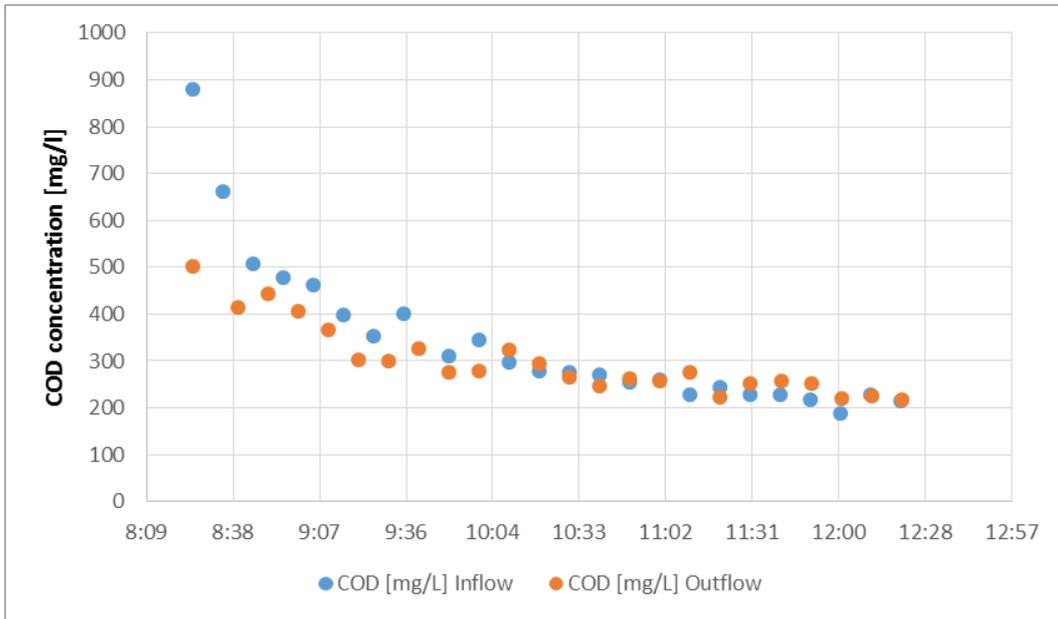
Figure 38 COD concentration during an exemplary dry weather test with a flow of 15 l/s (corresponding to a surface loading in the container of 1.6 m/h).
