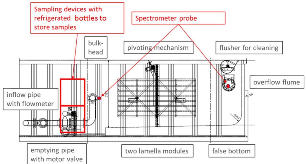
Figure 24 Position of sampling devices inside container.
