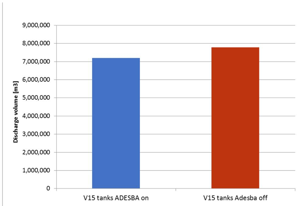
Figure 92 Total overflow volumes for a 10 year period. Results for four controlled CSOs in the catchment (scenario no. 15) with and with ADESBA.
