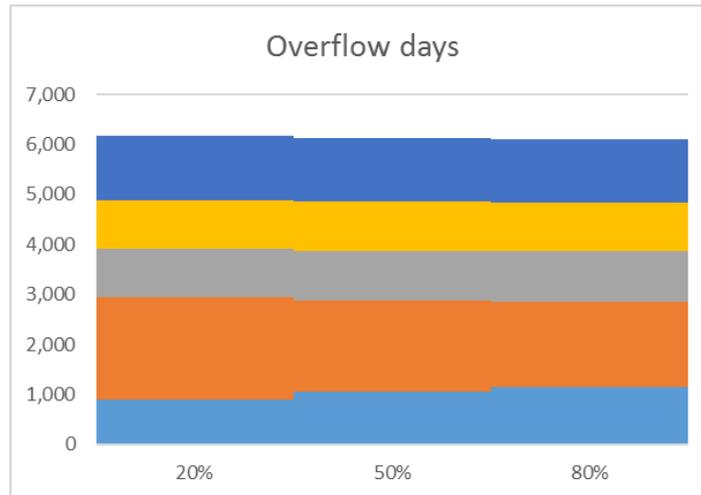
**Figure 69** Total overflow days resulting from the Simba# simulation with ADESBA in place. The throttle range in which ADESBA operates was varied from 20 to 50 to 80% of the total range between zero and Qmax. The simulations are based on 25 year MOMENT data. Different colours indicate overflow volume share of each CSO facility.
