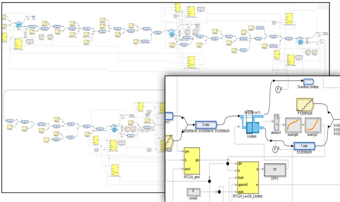
Figure 62 Structure of the network of the five CSO facilities to be controlled in Simba# including controllers.
