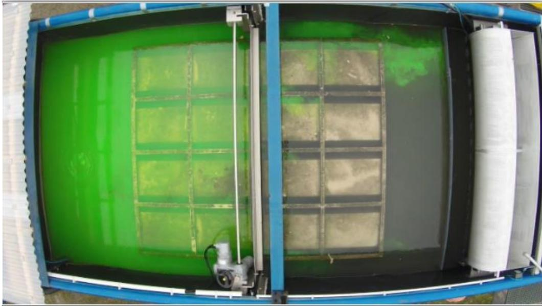
Figure 29 Aerial view of the container during the fluorescein tracer test. Flow direction is from left to right. A current bypassing the lamella modules on the left side was observed.
