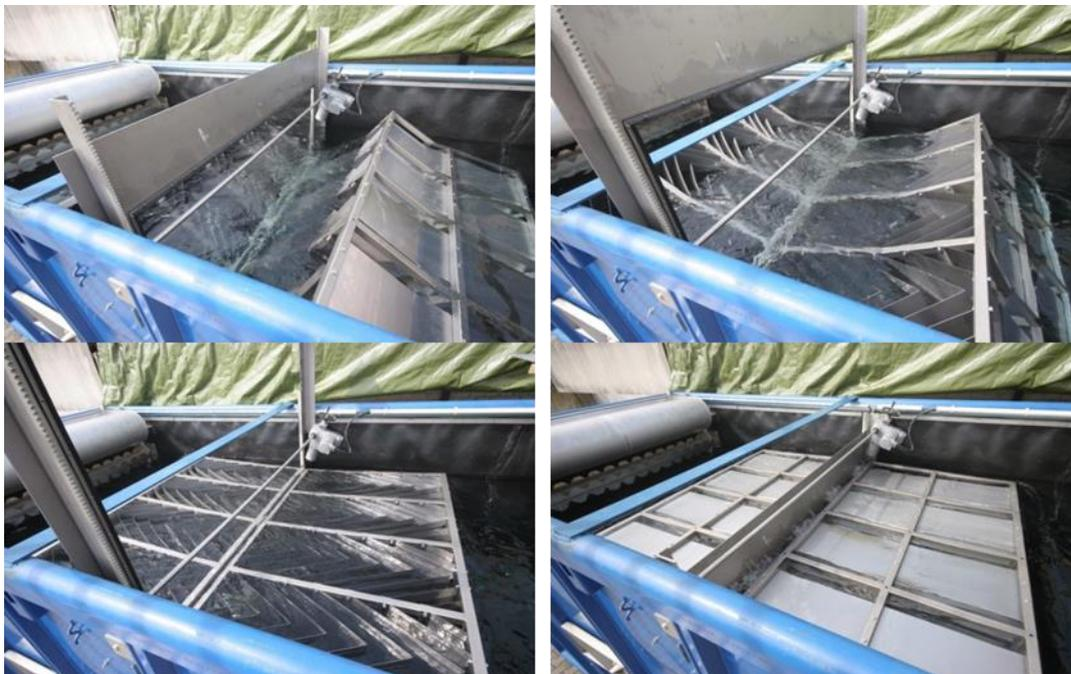
Figure 7 Self-cleaning process (here with clean water).
