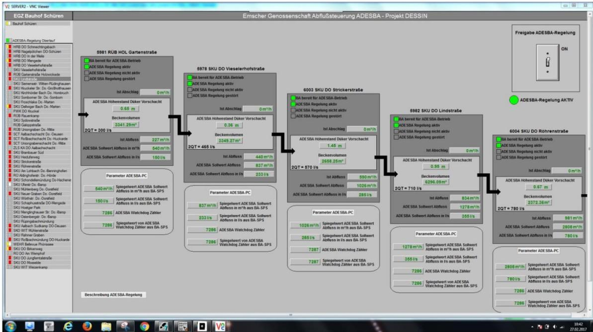
Figure 78 Newly developed overview of the total controlled system at the WinCC in the central office.
