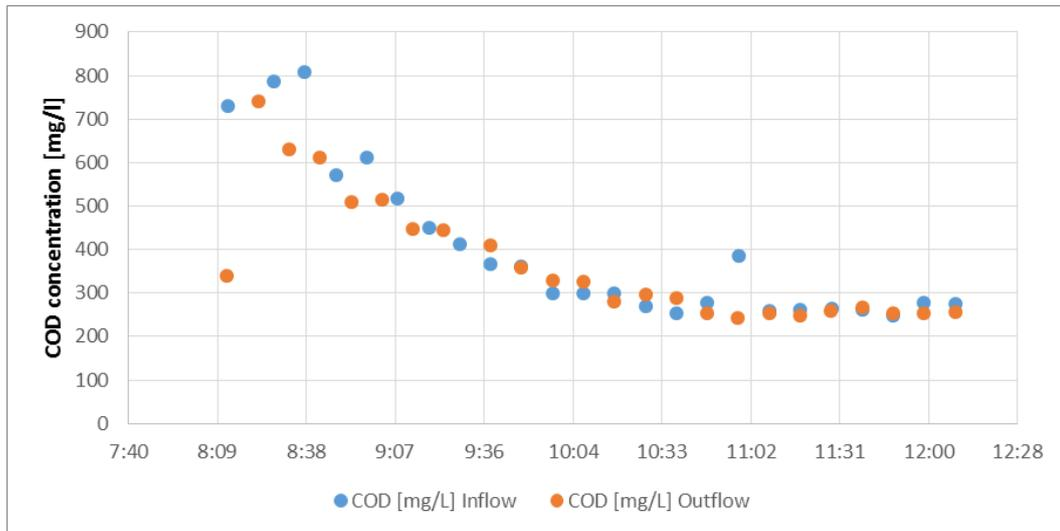
Figure 40 COD concentration during an exemplary dry weather test with a flow of 25 l/s (corresponding to a surface loading in the container of 2.7 m/h).
