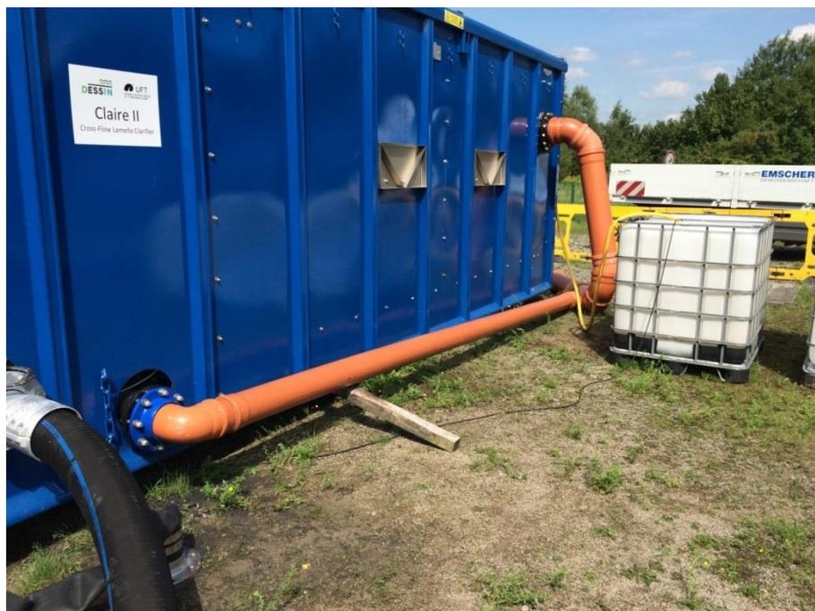
Figure 19 Optimization: Replacement of the flexible by a hard plastic emptying pipe connected to the discharge pipe, discharging into the next sewer.
