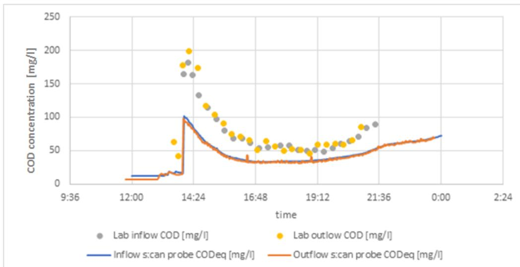
Figure 33 Comparison of COD concentration recorded with s::can probes (blue, orange) with those analyzed in the laboratory (grey, yellow).
