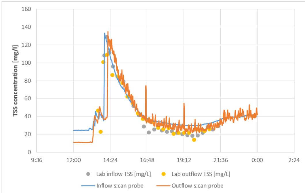
Figure 32 Comparison of TSS concentrations recorded with s::can probes (blue, orange) with those analyzed in the laboratory (grey, yellow).
