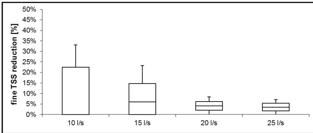
Figure 42 Reduction range for parameter fine TSS at different flow rates.
