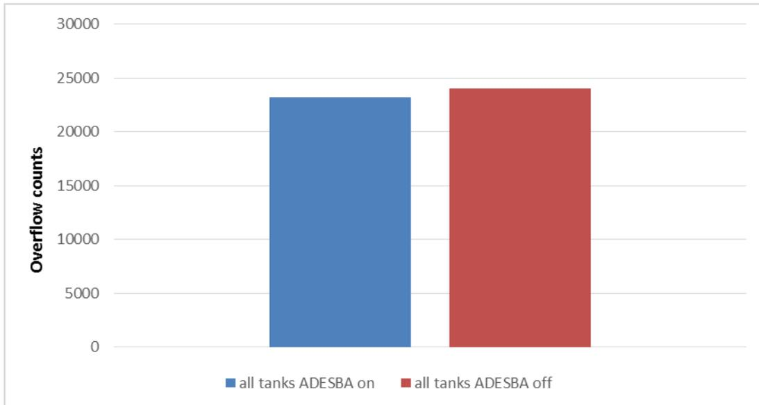
Figure 90 Total overflow counts for a 10 year period. Results for the whole catchment with and with ADESBA control.
