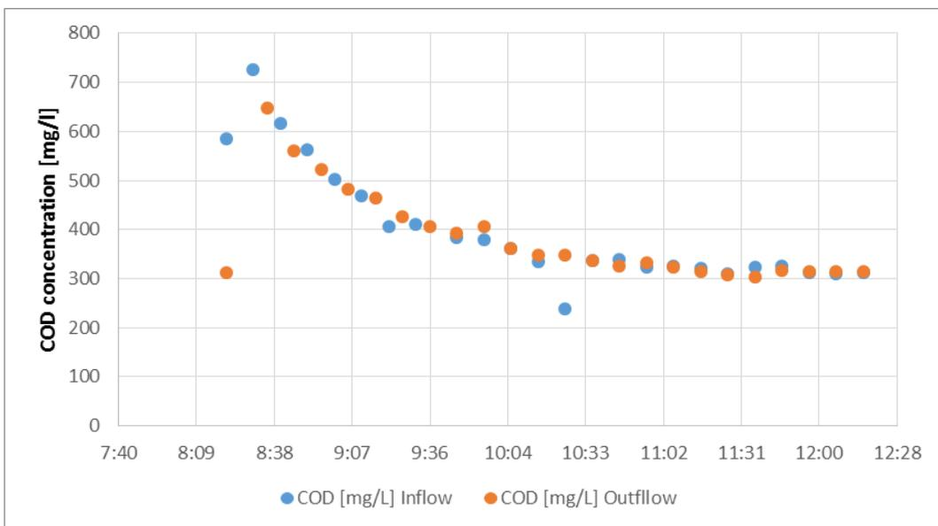
Figure 39 COD concentration during an exemplary dry weather test with a flow of 20 l/s (corresponding to a surface loading in the container of 2.2 m/h).
