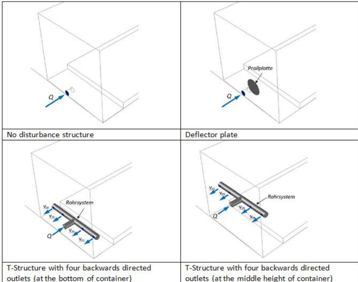
Figure 8 Different types of inlet structures to the test container.
