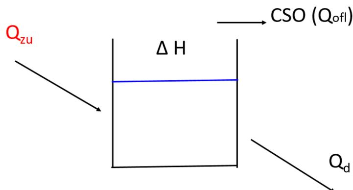
Figure 55 Parameters relevant for the calculation of the inflow ( $Q_{zu}$ ). The other three parameters ( $\Delta H$ ,  $Q_d$ ,  $CSO (Q_{ofl})$ ) are measured via sensors.  $\Delta H$  = water level,  $Q_{zu}$  = Inflow,  $Q_d$  = throttled outflow,  $CSO (Q_{ofl})$  = overflow.
