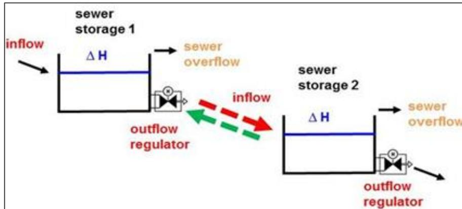
Figure 54 Overview of the real-time controlling mechanism of the ADESBA algorithm.  $\Delta H$  = water level.
