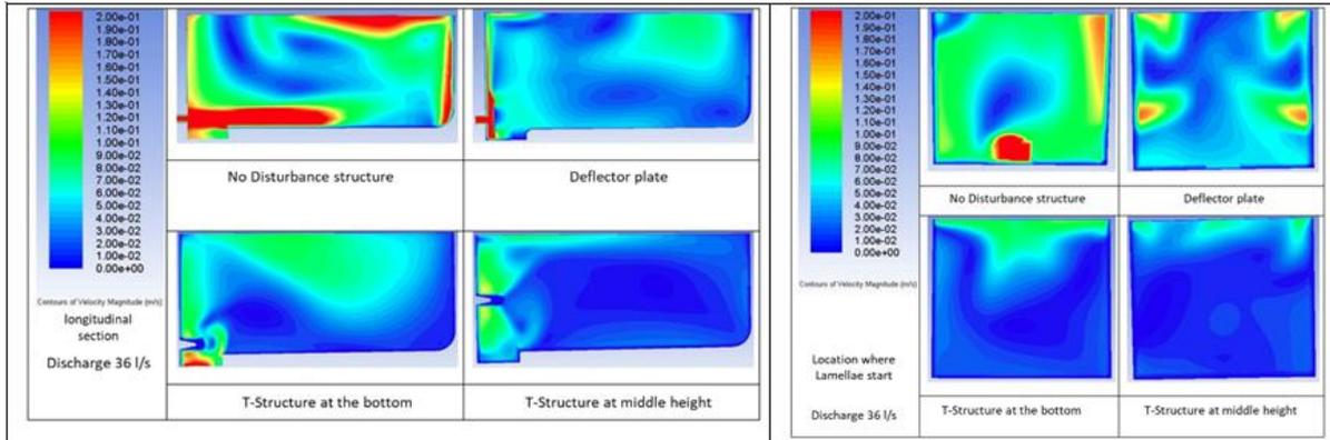
Figure 9 Modeled velocity distribution profiles inside the container at a discharge of 36 l/s. Left: Side view; Right: Cross section at beginning of lamella package.
