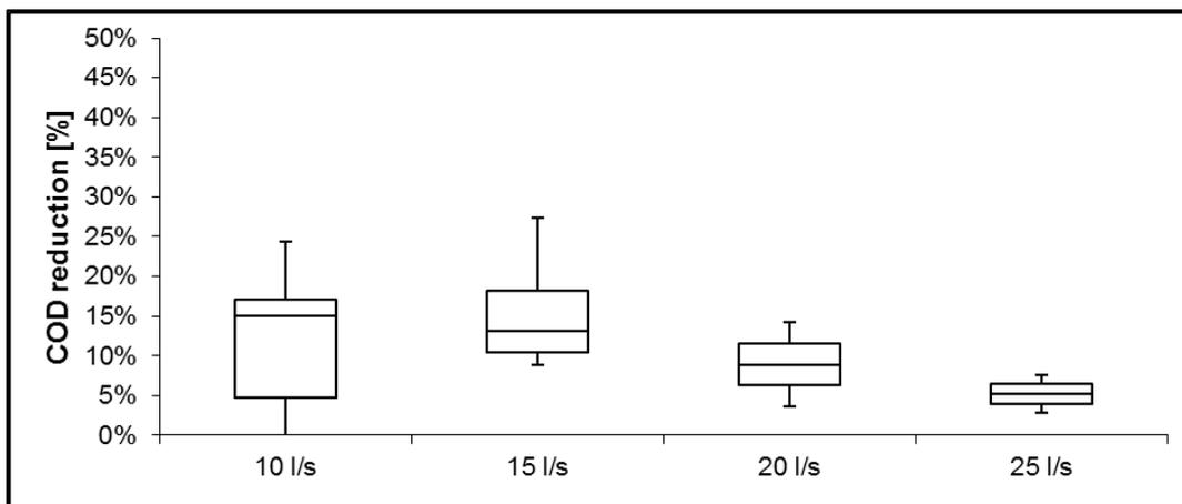
Figure 43 Reduction range for parameter COD at different flow rates.
