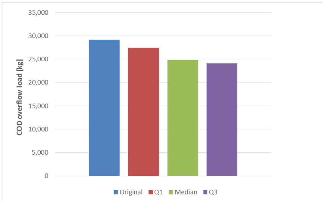
Figure 52 Theoretical COD load in the overflow of CSO Gartenstraße in one year (2014). “Original” refers to the overflow without lamellae, “Q1”, “Median” and “Q3” represents the overflow with lamellae (storage volume equipped with lamellae by 50 %) modelled with the 25<sup>th</sup>, 50<sup>th</sup> and 75<sup>th</sup> percentile of the efficiencies determined in the container test, respectively.
