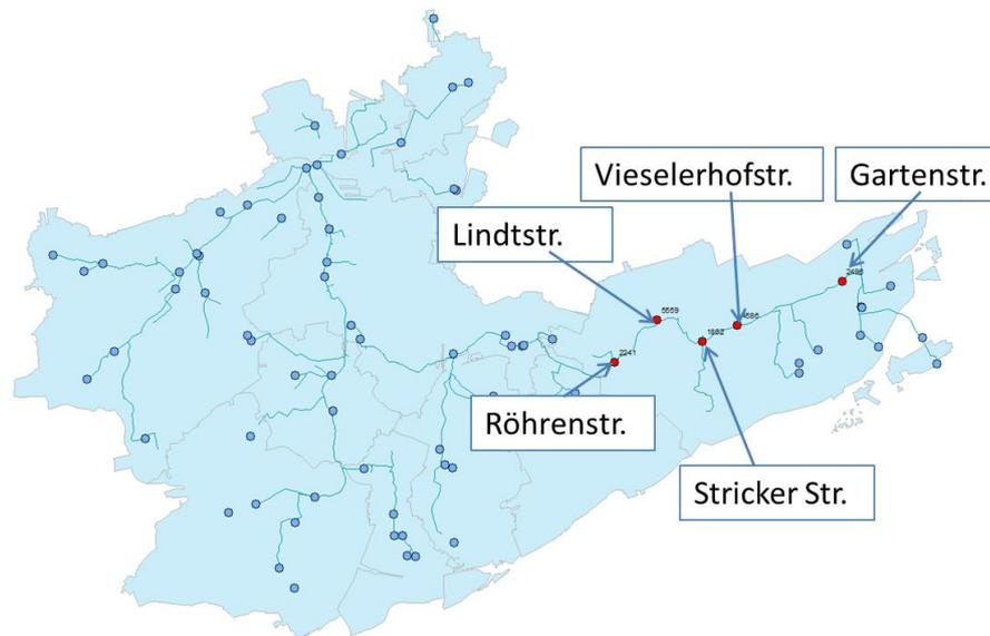
Figure 57 Network of the five CSO facilities in the Emscher sub-catchment of Dortmund Deusen to be real-time controlled.
