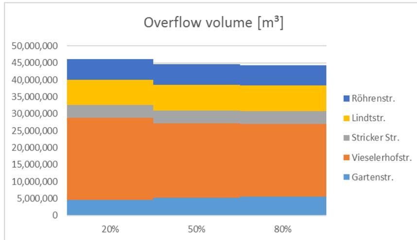
**Figure 67** Total overflow volume resulting from the Simba# simulation with ADESBA in place. The throttle range in which ADESBA operates was varied from 20 to 50 to 80% of the total range between zero and Qmax. The simulations are based on 25 year MOMENT data. Different colours indicate overflow volume share of each CSO facility.
