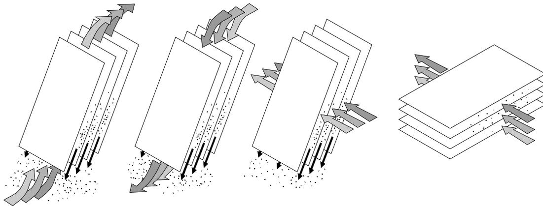
Figure 2 Upflow, downflow, cross-flow and horizontal plate settlers (from left to right) (Weiss2014).
