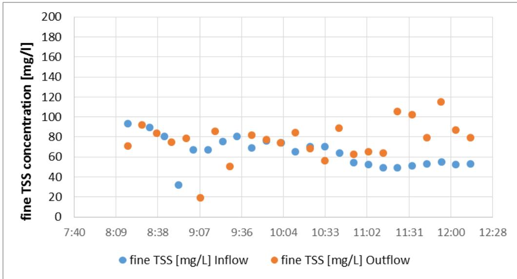
Figure 35 Fine TSS concentration during an exemplary dry weather test with a flow of 10 l/s.
