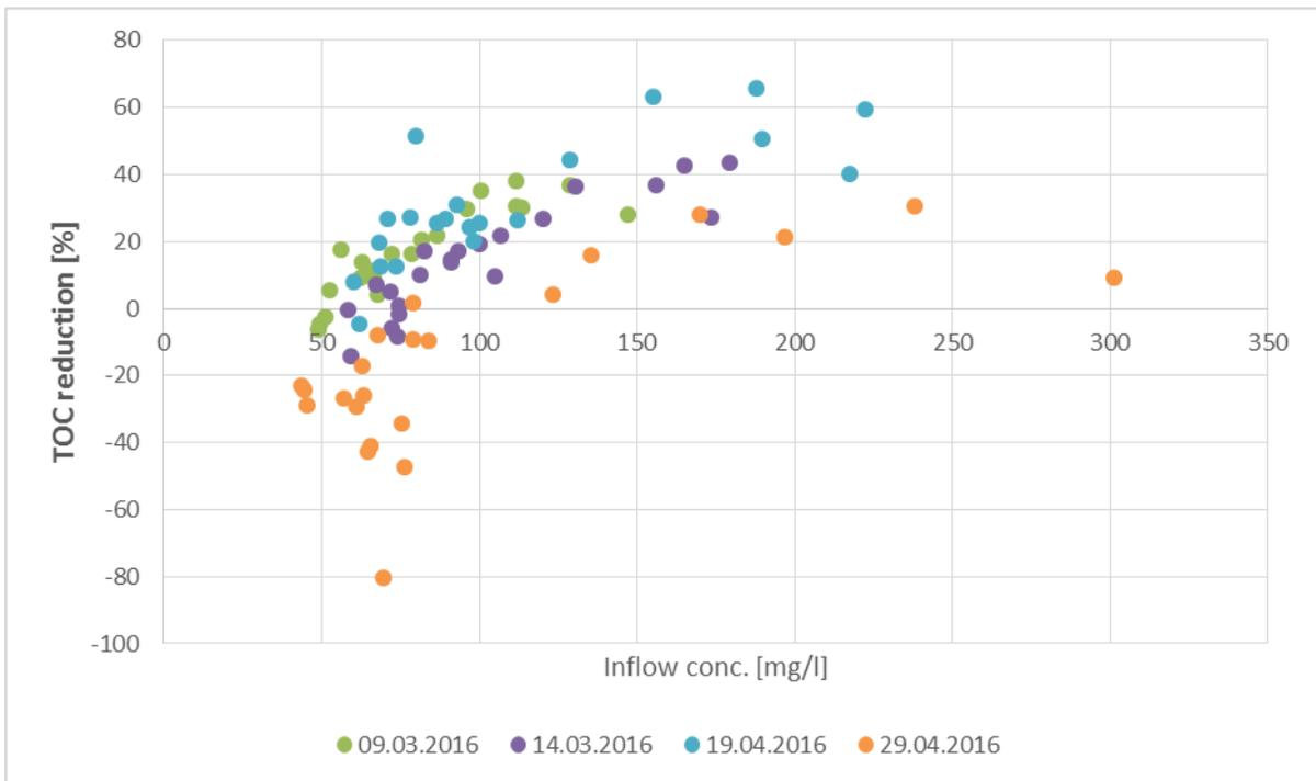
Figure 48 Concentration of TOC in the inflow and reduction on the way to the overflow for four test runs with dry weather at a flow rate of 10 l/s.
