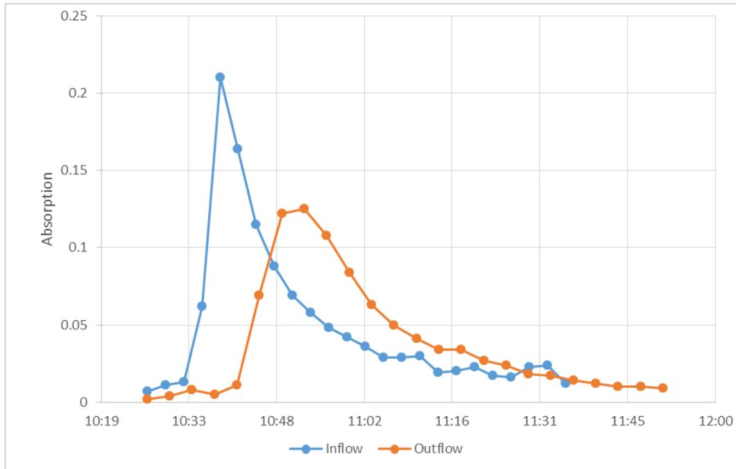
Figure 30 Results of one Fluorescein tracer test at a discharge of 10 l/s. The lag time identified between the inflow and overflow peak is 13 minutes.
