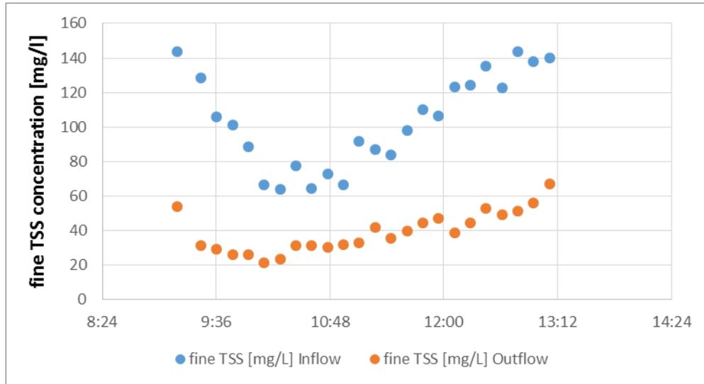
Figure 49 Fine TSS concentration during an exemplary dry weather test without lamellae with a flow of 10 l/s.
