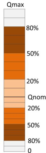
Figure 66 Throttle range, *i.e.* valve opening/closing from the nominal throttle flow towards Qmax and towards zero discharge (%).
