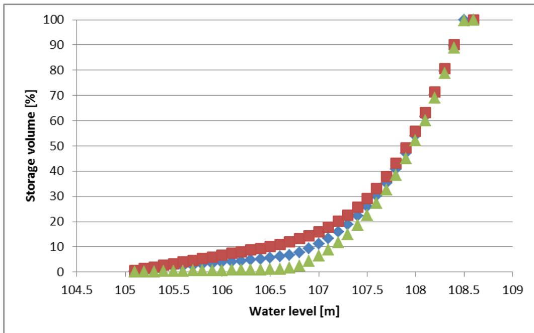
Figure 71 Exemplary scenario for over- and underestimating the water-level-to-storage-volume relationship (red and green, respectively) at CSO Vieselerstr. The blue line is indicating “real” conditions.
