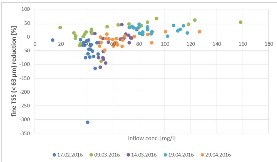
Figure 46 Concentration of fine TSS in the inflow and reduction on the way to the overflow for five test runs with dry weather at a flow rate of 10 l/s.
