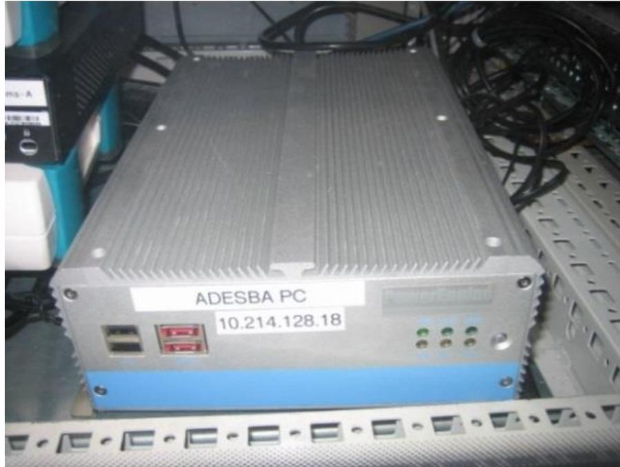
Figure 75 ADESBA-PC installed in the central control office Bauhof Schüren in Dortmund.
