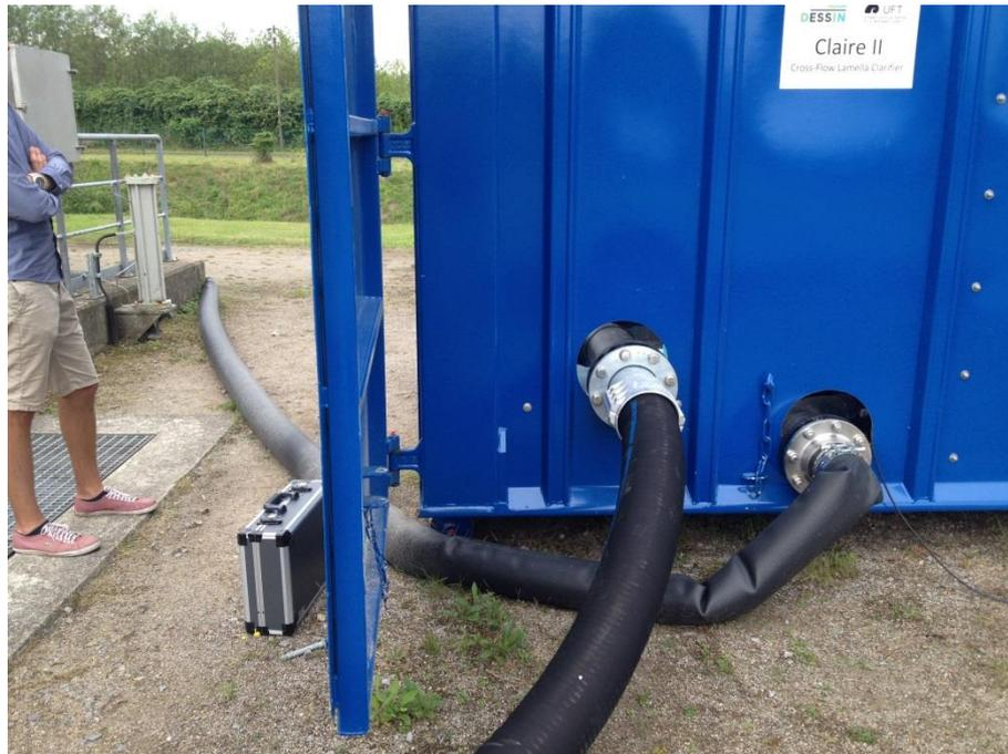
Figure 18 Attachment of a flexible emptying pipe, discharging back into the pump sump.
