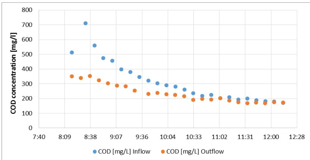
Figure 36 COD concentration during an exemplary dry weather test with a flow of 10 l/s.
