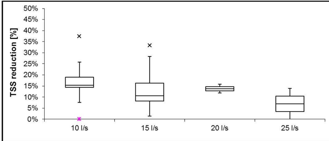
Figure 41 Reduction range for parameter TSS at different flow rates.
