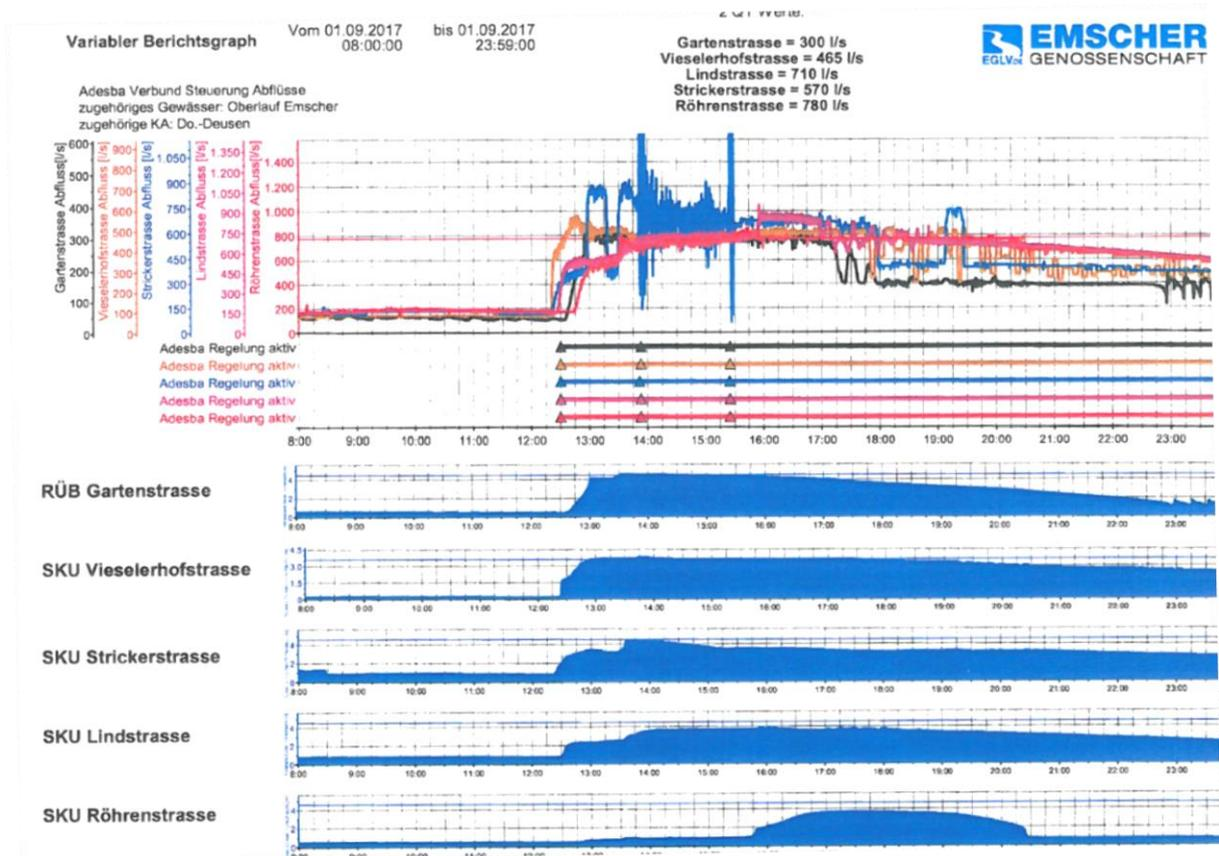
Figure 81 Graphical report from ACRON visualizing the outflow and filling level in all five CSOs on 1st September 2017.
