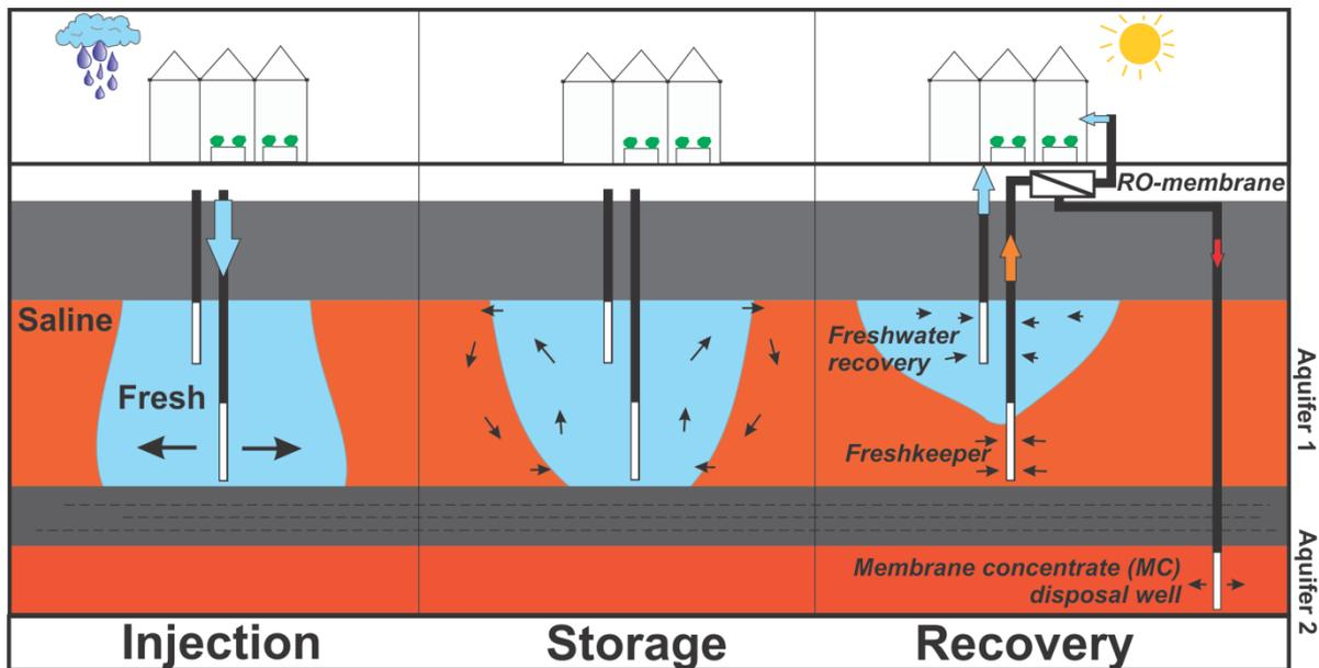
Figure 8: Locations of the groundwater abstractions for desalination: BWRO at the (lateral) fringe of the injected freshwater bubble, ASRRO below the injected freshwater bubble.
