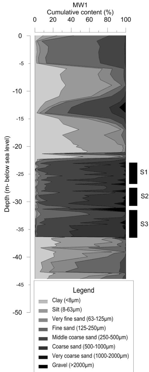
Figure 7: Cumulative grain size contents observed at MW1 (at 5 m from ASR well 1). S1-S3 mark the depth intervals of the ASR well screens.
