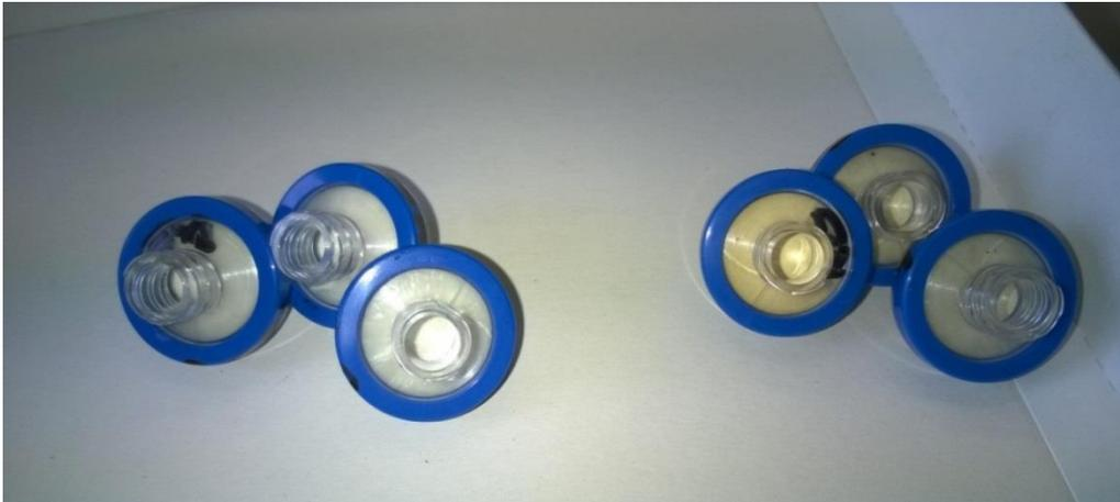
Figure 9: The Convergence MFI/SDI 0.45 micron filters used to derive the MFI/SDI of the ASRRO feed water (left) and the BWRO feed water (right) (date: June 19, 2015).
