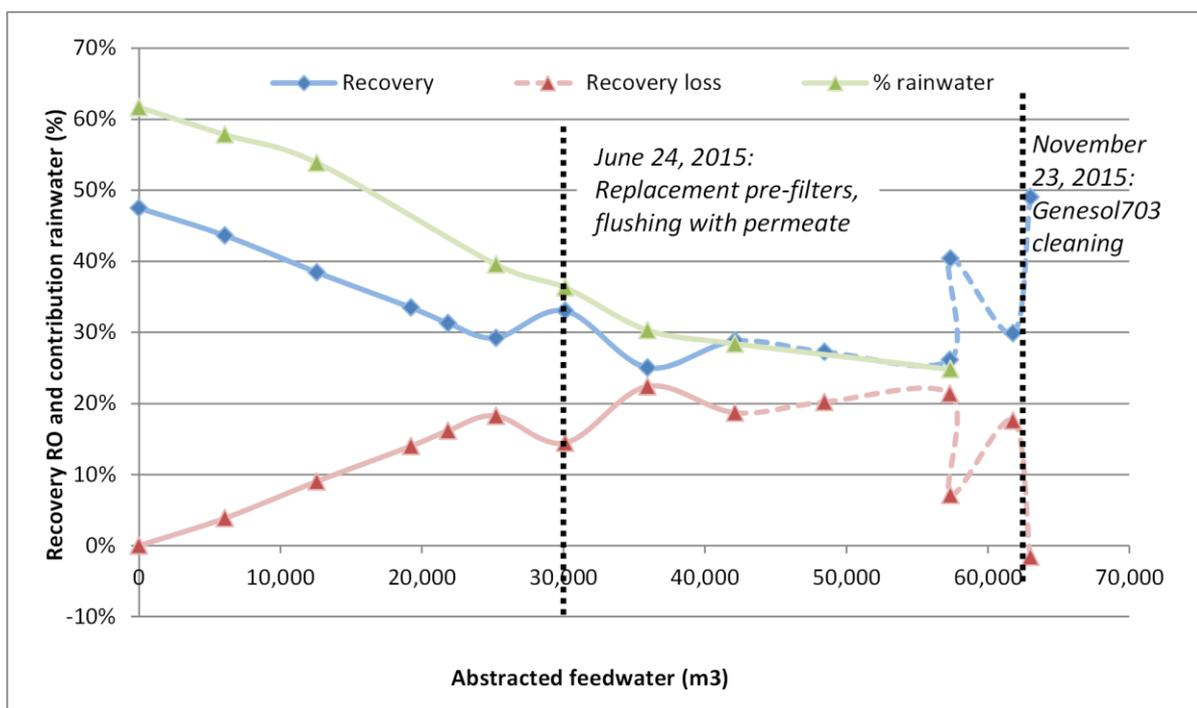
Figure 14: Recovery and recovery loss of the BWRO membranes, and the contribution of rainwater to the RO-feed water in 2015. Solid lines indicate continuous operation, dashed lines indicate frequent periods of standstill and flushing alternating with irregular operation.
