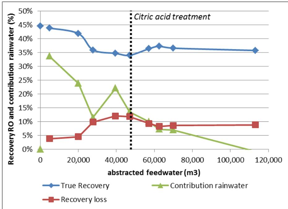
Figure 11: Recovery achieved by the BWRO-plant ('true recovery'), contribution of rainwater to the feed water. At abstracted feed water = 0 m3, the operational data of the last servicing round (June 20, 2012) is shown. At this time, the installation had his normal design capacity.
