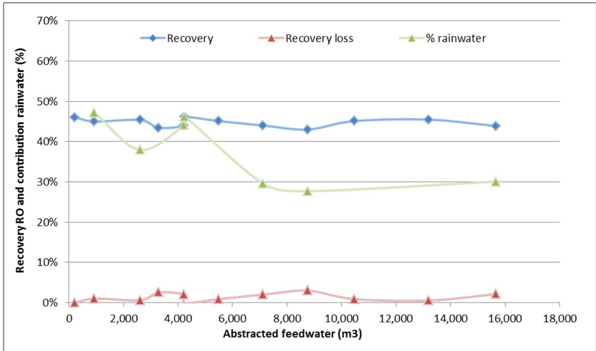
Figure 16: Recovery and recovery loss of the ASRRO-plant and the contribution of rainwater to the ASRRO-feed water in 2015.
