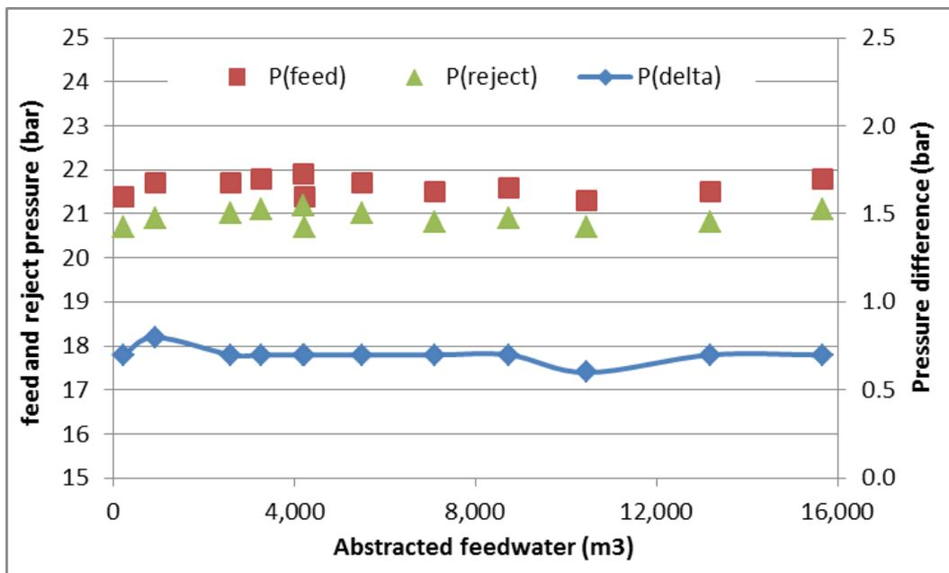
Figure 17: Feed and reject pressures at the ASRRO-plant in 2015.
