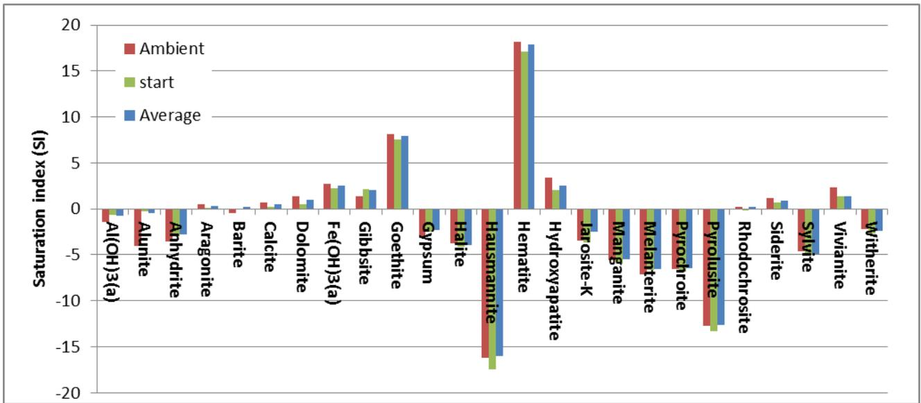
Figure 12: Saturation indices of minerals in the BWRO feed water based on the composition of the brackish water and the feed water composition at the start of abstraction and the average composition in 2013.
