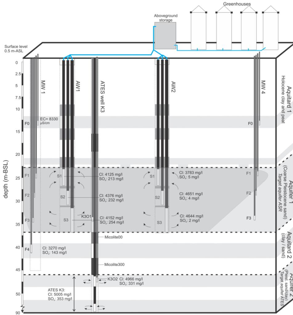
Figure 6: Cross-section of the Westland ASR-pilot, including the ambient groundwater quality observed prior to the ASR operation.
