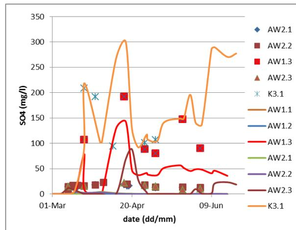
Figure 13: Modelled and observed  $\text{SO}_4$ -concentrations at the most relevant well screens.
