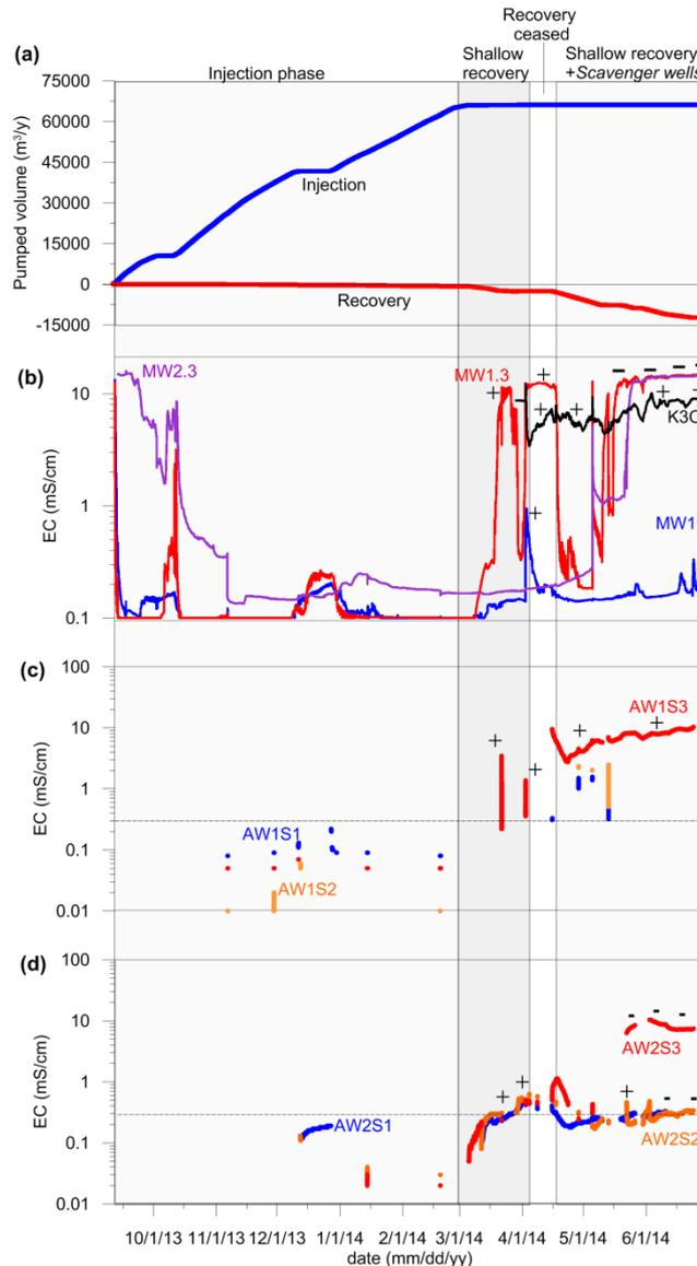
**Figure 12:** Pumping of the ASR system during Cycle 2 in 2013/2014 (a), EC observations at MW1 at 5 m from AW1 (b), and the EC in the recovered water at AW1 (c) and AW2 (d). AW2.1 and AW2.3 were used for freshwater recovery (12,324 m<sup>3</sup>). Presence of increased SO<sub>4</sub>-concentrations (deep saltwater from Aquifer 2) are marked by '+', while its absence is marked by '-' (indicating shallow saltwater from Aquifer 1).
