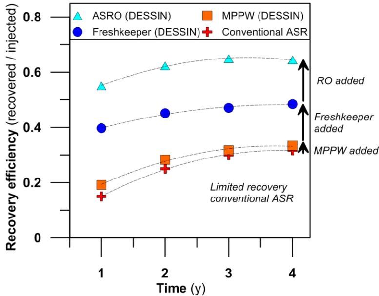
Figure 1: Most relevant results of the SEAWAT modeling study: an increase in recovery efficiencies at the Westland target aquifer thanks to the introduction of the MPPW, the Freshkeeper, and ASRRO.
