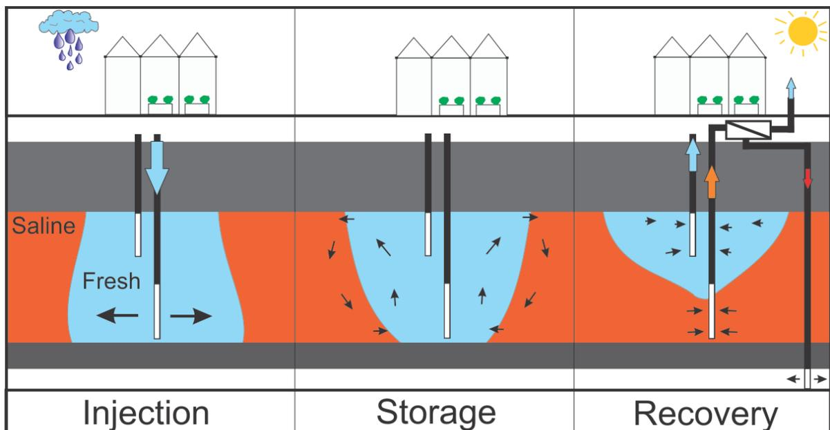
Figure 4: The introduction of the MPPW for deep injection and shallow recovery in combination with a Freshkeeper and optional RO-treatment for a maximal recovery of freshwater (ASRRO).
