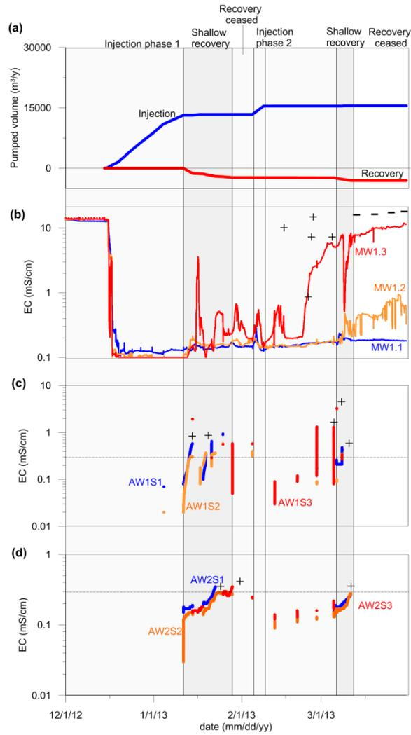
Figure 10: Pumping of the ASR system during cycle 1 in 2012/2013 (a), EC observations at MW1 at 5 m from AW1 (b), and the EC in the recovered water at AW1 (c) and AW2 (d).
