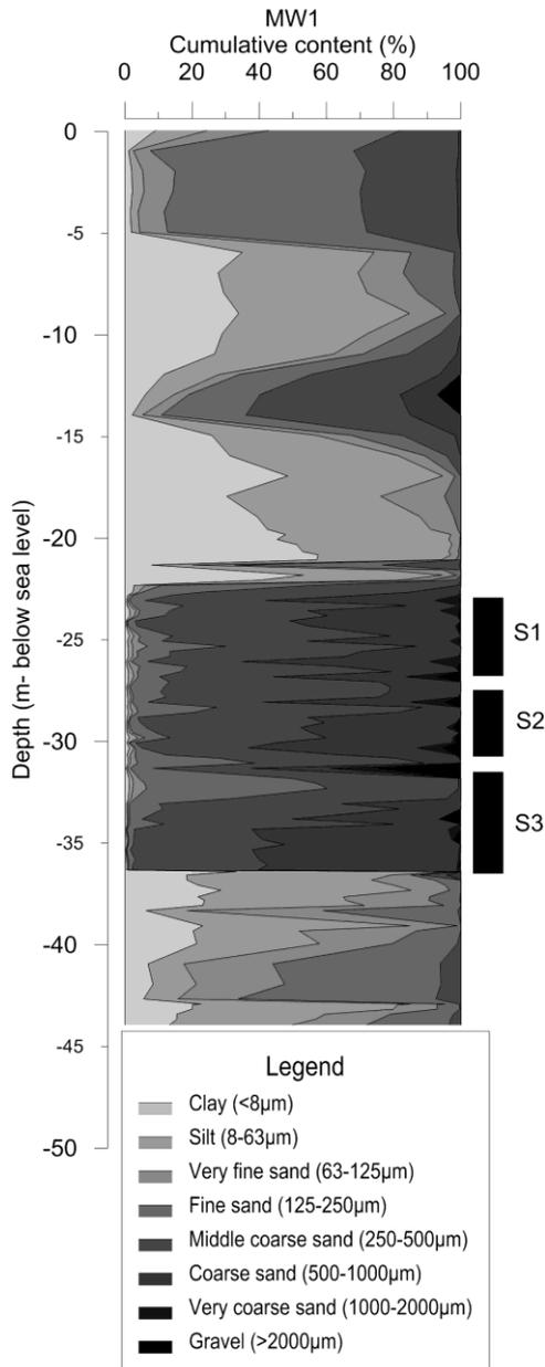
Figure 8: Cumulative grain size contents observed at MW1 (at 5 m from ASR well 1). S1-S3 mark the depth intervals of the ASR well screens.
