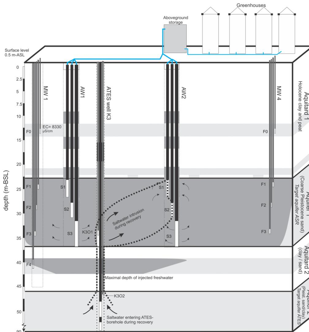
Figure 15: Deep saltwater intrusion via a borehole during recovery of injected freshwater at the Westland ASR site.
