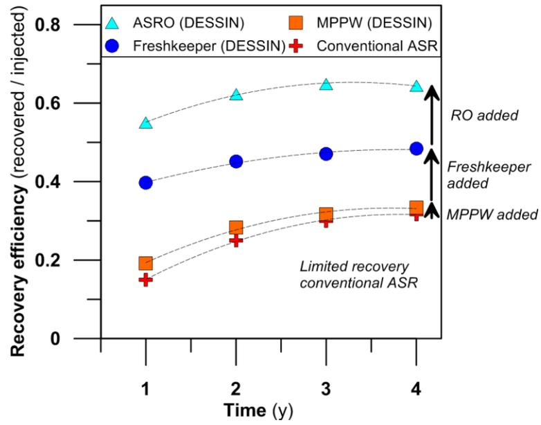
Figure 18: Most relevant results of the SEAWAT modelling study: an increase in recovery efficiencies at the Westland target aquifer thanks to the introduction of the MPPW, the Freshkeeper, and ASRRO.
