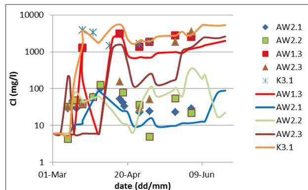
Figure 14: Modelled and observed  $\text{Cl}$ -concentrations at the most relevant well screens.
