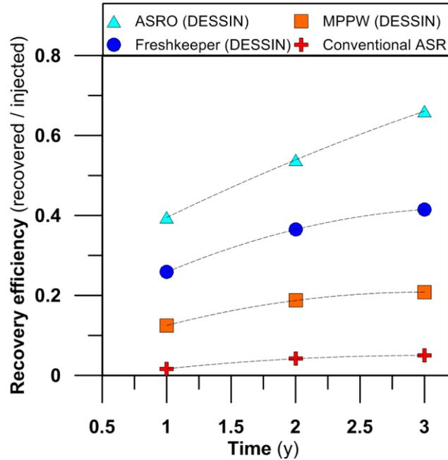
Figure 17: Recovery efficiencies at the Westland ASR site assuming a doubled target aquifer thickness resulting from the SEAWAT groundwater transport model for a conventional ASR well (one well screen, fully penetrating), multiple partially penetrating wells without a 'Freshkeeper' (scenario MPPW), for a MPPW in combination with a 'Freshkeeper' (scenario Freshkeeper), and for a scenario in which RO is applied on the intercepted brackish water to produce additional freshwater (50% of the flux).
