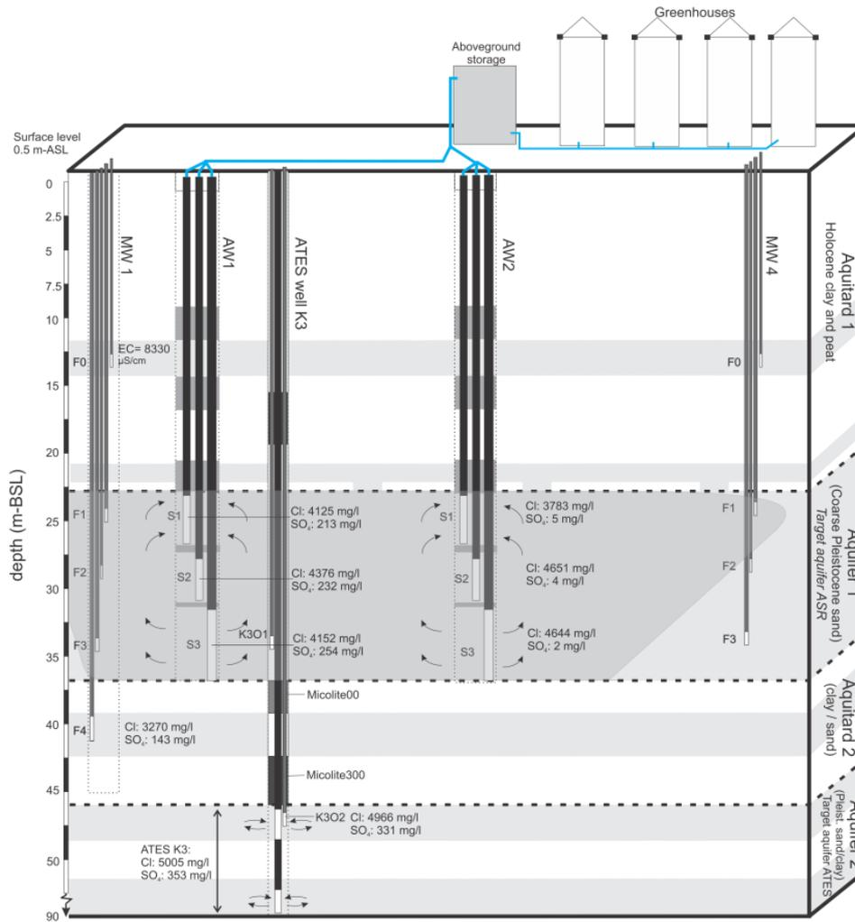
Figure 6: Cross-section of the Westland ASR-pilot, including the ambient groundwater quality observed preceding the ASR operation.
