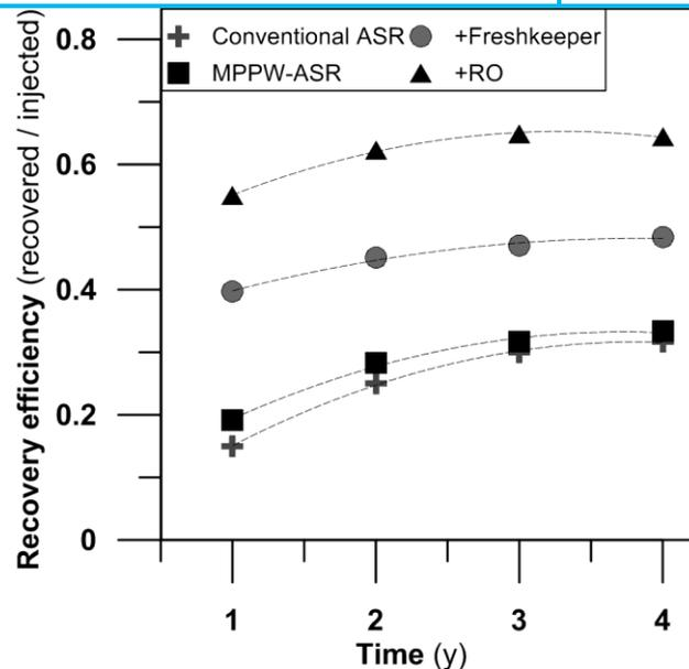
**Figure 16:** Recovery efficiencies at the Westland ASR site without the borehole leakage resulting from the SEAWAT groundwater transport model for a conventional ASR well (one well screen, fully penetrating), multiple partially penetrating wells without a ‘Freshkeeper’ (scenario MPPW-ASR), for a MPPW in combination with a ‘Freshkeeper’ (scenario +Freshkeeper), and for a scenario in which RO is applied on the intercepted brackish water to produce additional freshwater (50% of the flux).
