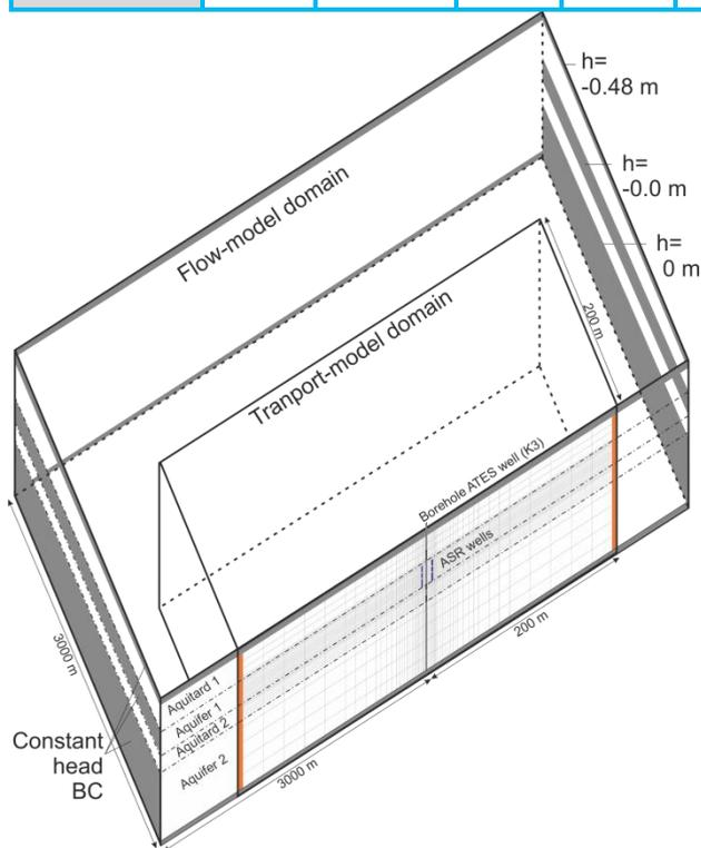
Figure 9: Set-up of the Westland ASR groundwater transport model (half-domain).
