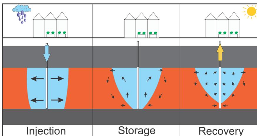
Figure 3: Freshwater loss during ASR in brackish and saltwater aquifers due to buoyancy effects.
