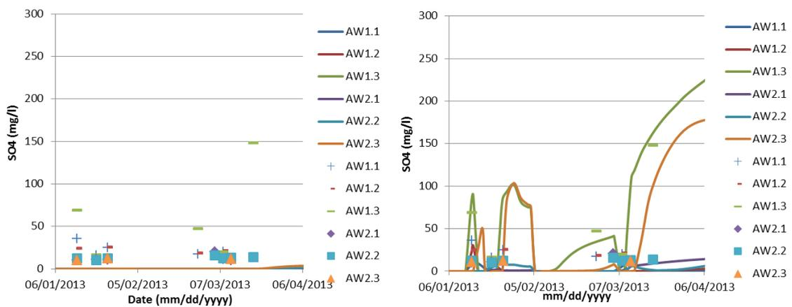
Figure 11: Modelled (solid lines) and observed (data points) SO<sub>4</sub>-concentrations. High concentrations indicate admixing of deeper saltwater. Left = no borehole leakage, right = borehole leakage via a 1x1 m borehole with K=1000 m/d).
