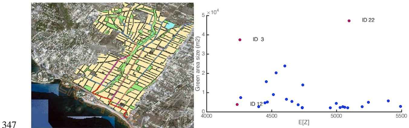
**Figure 6:** Urban area with alternative locations of sewer-mining installation (left panel), evaluation of alternative locations with Monte-Carlo simulation (right panel).
