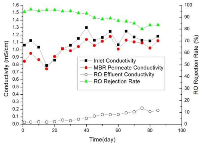
Figure 10: Conductivity data retrieved by the installed sensors.
